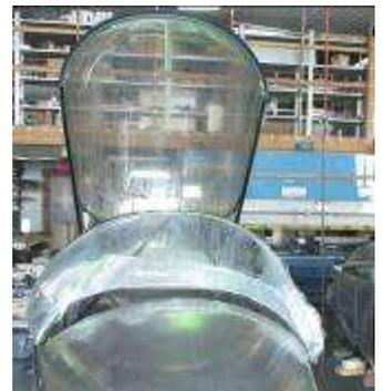
Allow 1/8" clearance of the front edge with the fuselage when the canopy is open.
