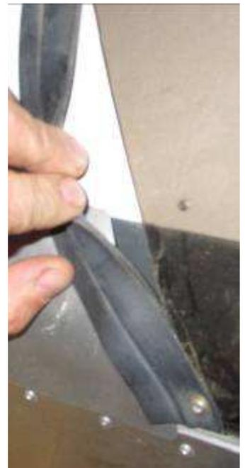
Leave at least 7mm between the aft edge and the bubble.
