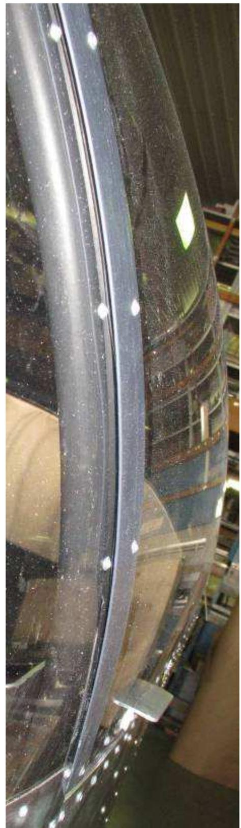
No gap on the front side. It is acceptable for the strip not to touch the rear canopy.
