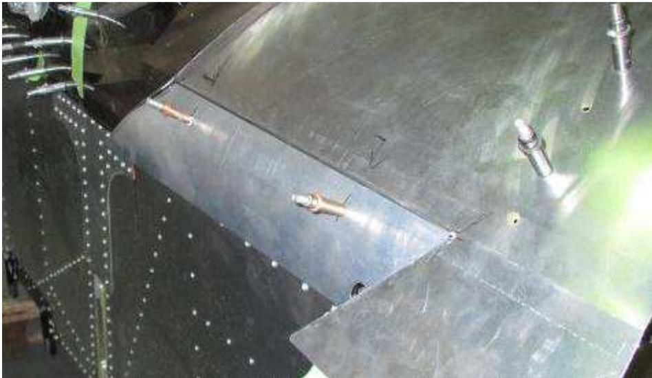
Line up the top edge. Trim the front and aft ends. Drill the hole for the bolt (big enough to insert a socket).
