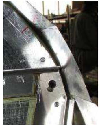
Flatten the bend, the bend tends to leave a gap at the firewall
