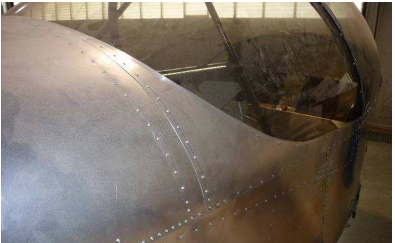
Alternative: installation of the rear canopy skin 65C3-9 with a separate rivet line
