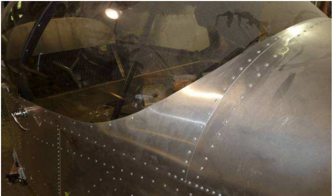
Alternative: installation of the rear canopy skin 65C3-9 with a separate rivet line
