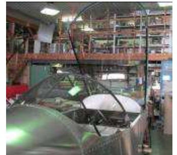
Wait to secure the front canopy to the tube frame until the strip is installed.
