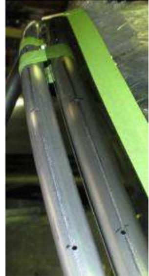
Position the front canopy on the fuselage. Line up the aft edge between the 2 tubes.
