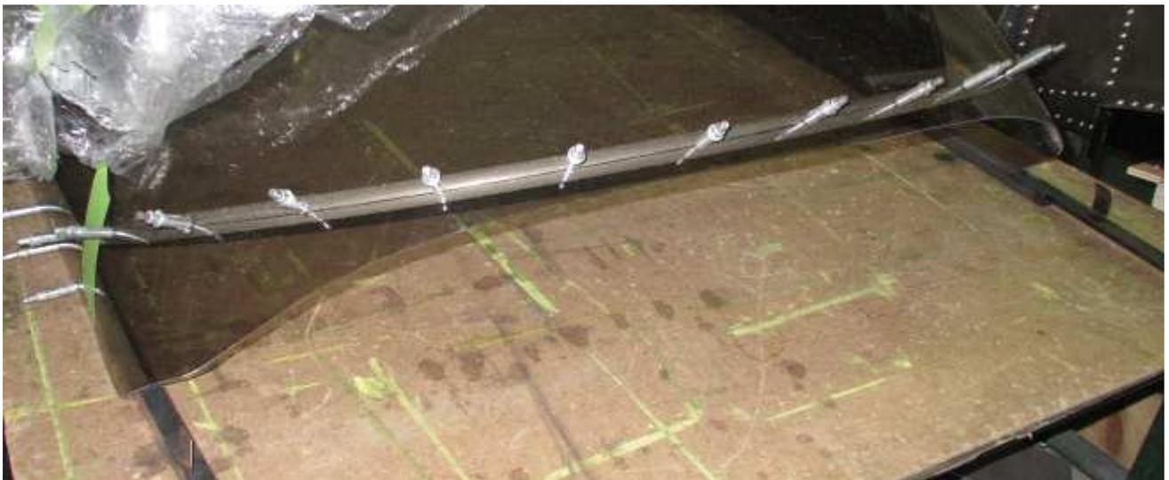
Mark the aft edge of the FRONT CANOPY FRAME GUSSET 65C3-12 on the side frame (left and right side).
