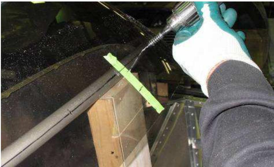
Using the drill to mark the holes with a shallow dimple.
