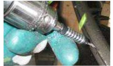
Mark the pre-drilled holes in the tube on the bubble. Use a #40 drill to drill a small impression over the existing holes - do NOT drill through.
