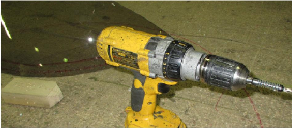
**IMPORTANT:** Use a wood block on the back-side to drill a clean, shatter-free hole.
