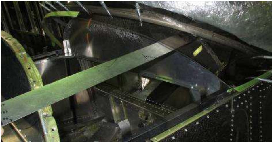
Keep trimming the front edge until it does not touch the strip.
