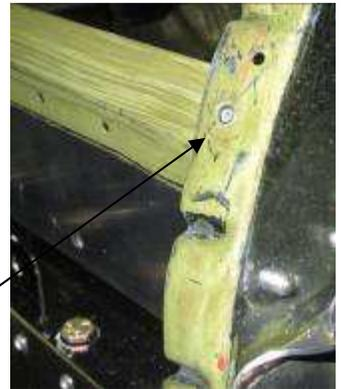
Flush rivet at front through firewall flange
