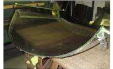
Remove the bubble to drill the 5/32" holes in the rear tubes.
