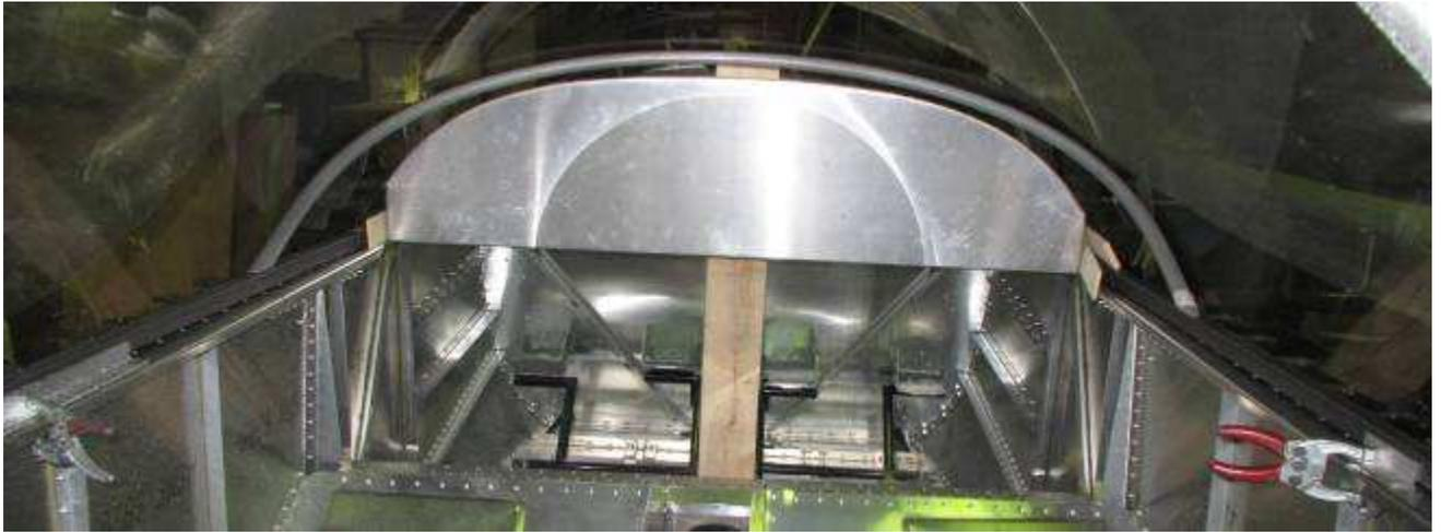
Check that the tube is centered over the instrument panel (left and right sides are equal)
