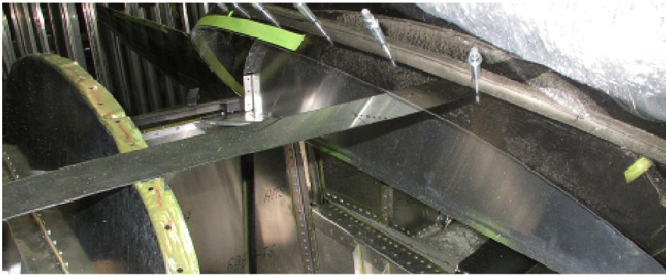
Flexible edge between instrument panel and firewall.
