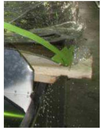
To cut the canopy on the fuselage, raise the canopy with a board across the fuselage.
