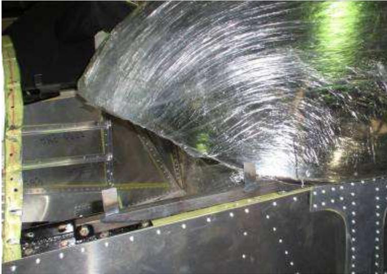
The front corner is approximately 20mm forward of the instrument panel
