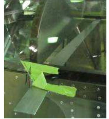
Slide a strip across fuselage to the support the front edge of the canopy
