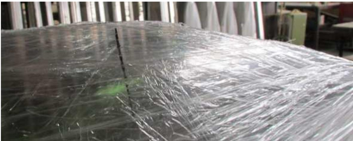
Rear right mark. The shorter perimeter distance is the front. When looking at the bubble from the side, note the front bottom edge is cut on a steeper angle than the slope at the rear.
