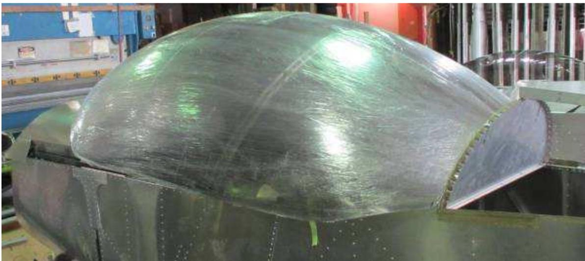
Let the back the bubble overhang on the outside of the fuselage.
