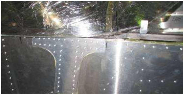
Mark the location of the weld with a vertical line. Mark the cut even with the top of the canopy side frame
