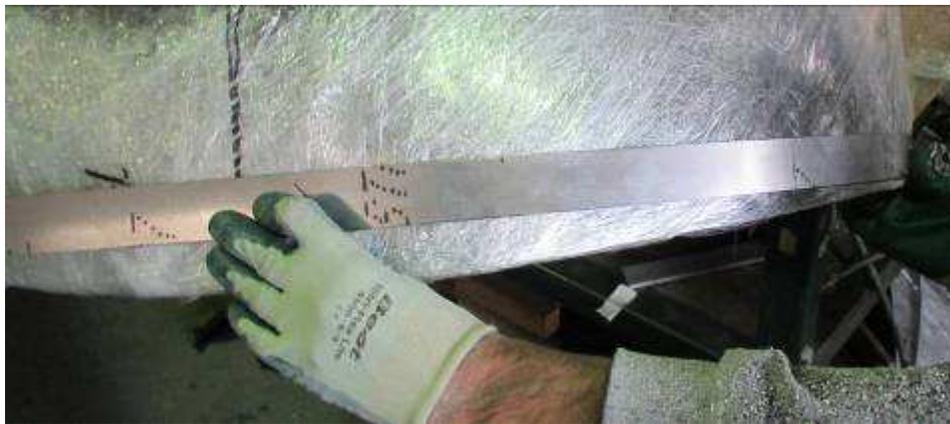
Flexible straight edge to connect the 3 points along the front of the bubble.
