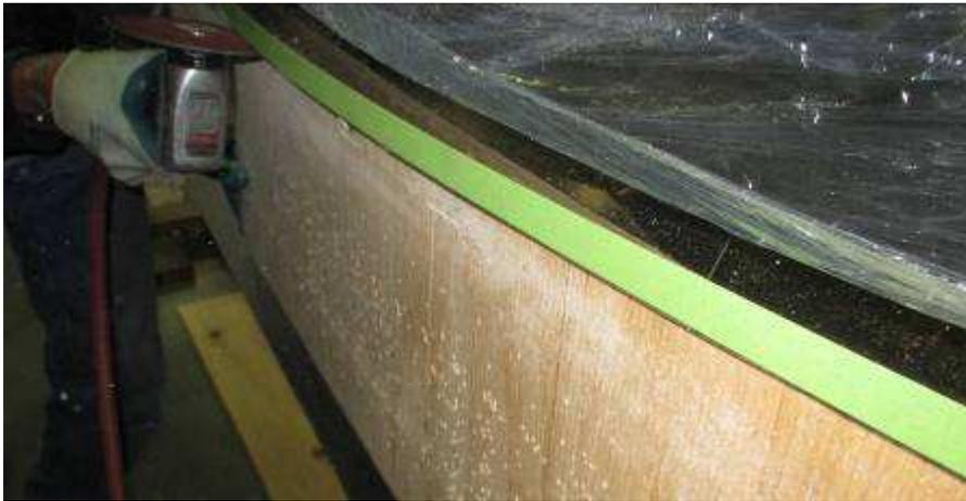
Trim the sides even with the top of the fuselage.
