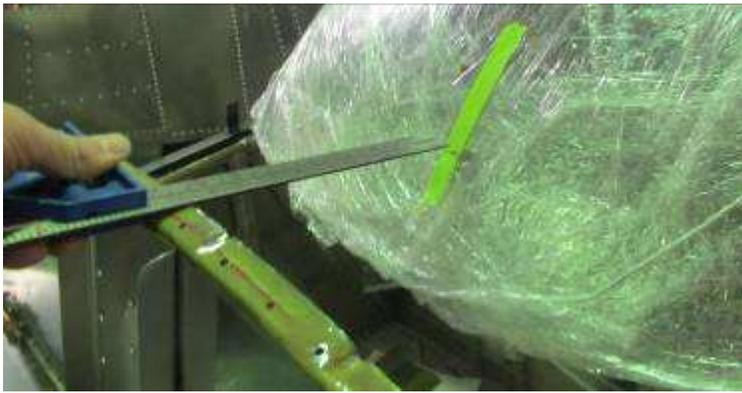
Push the left and right sides of the bubble against the side frame, sight across the firewall and instrument panel and mark a point approximately 40mm below the top skin on the aircraft center line.
