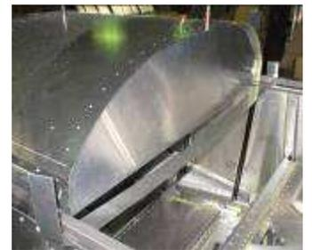
Support strip (positioned on the cabin-side of the instrument panel) to keep the front edges of the bubble even with top of the fuselage sides.
