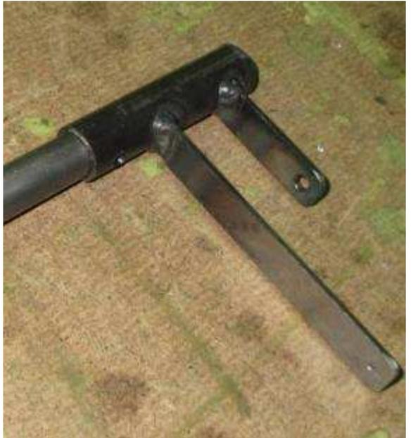
25mm overlap - insert the ends on the tube - make sure there are no burrs inside the tubes -
