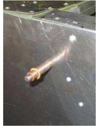
**From the inside, drill the front bottom hole in the bearing. Cleco from the outside.**
