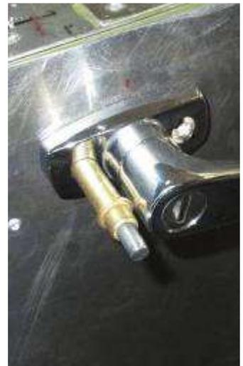
**Position the handle and drill the front hole through the bearing.**
