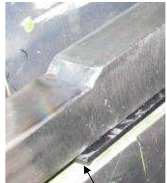
Clearance, Check that when the latch is closed the parts do not touch.
