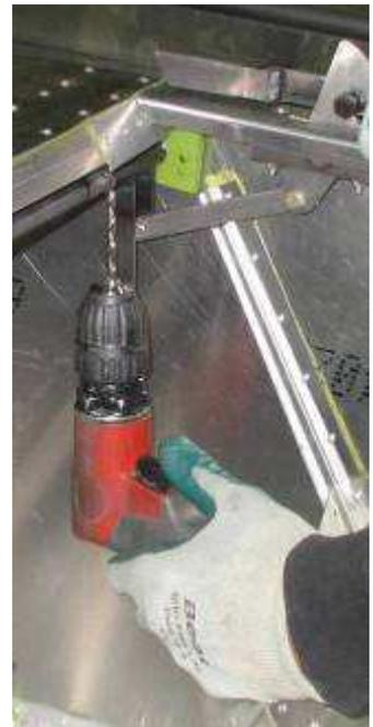
**Back drill through the pre-drilled holes in left and right tubes.**
