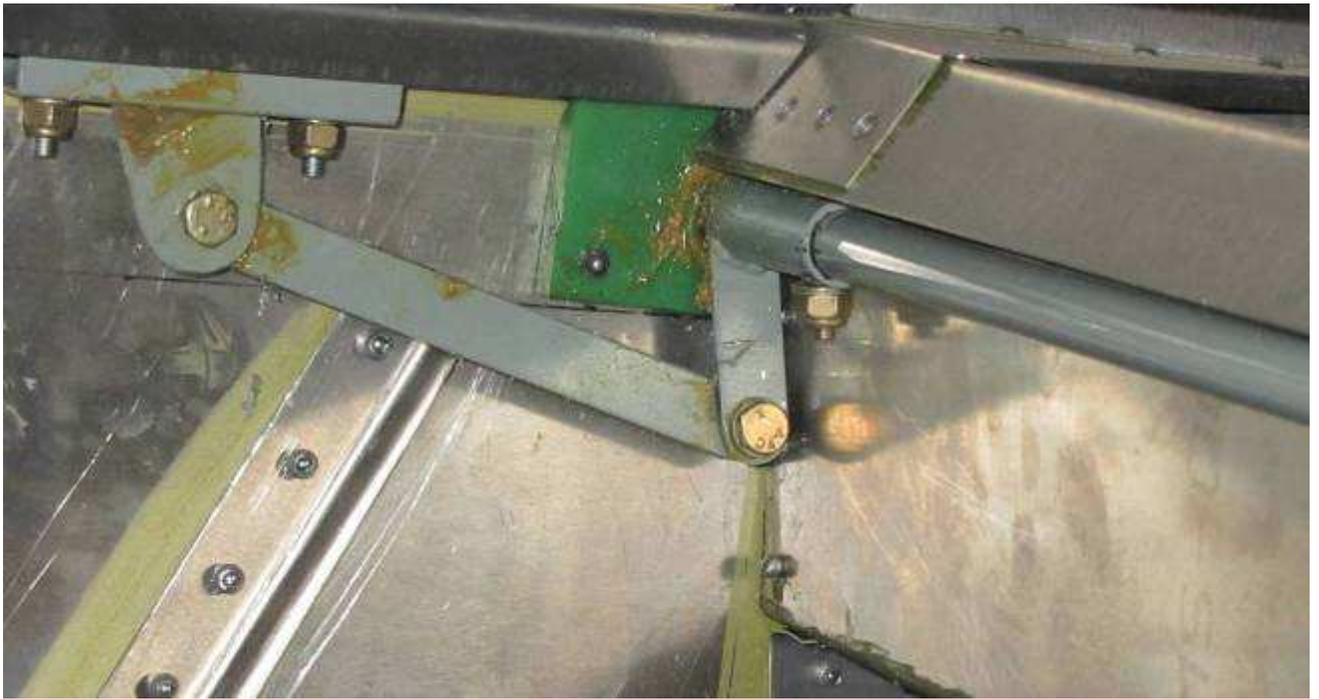
Paint the steel parts and re-assemble with bolts.
