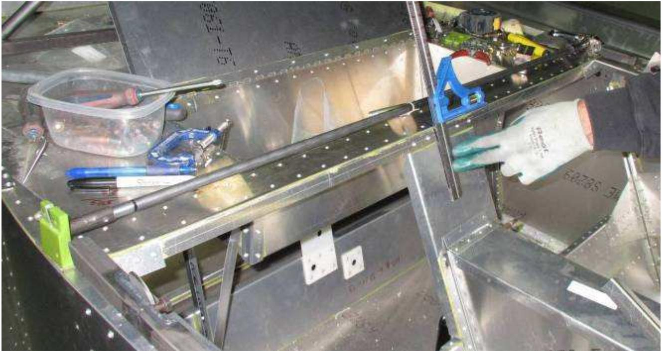
Use a square to mark the position of the handle on the channel
