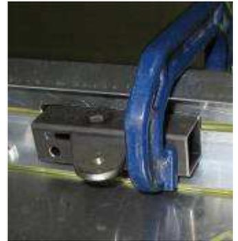
Check that the latch is pushed against the rivets in the side skin.
