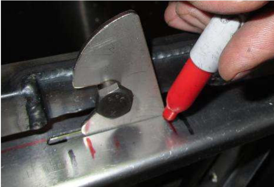
Mark the position of the latch in the close position
