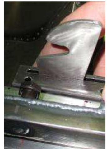
Open the latch and mark the aft edge. The length of the slot is between the closed and open position.
