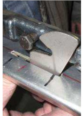
Check that the slot is long enough to swing the latch open.
