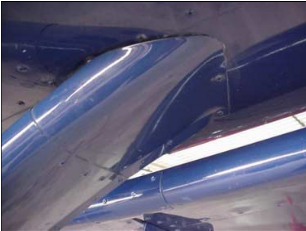
Two A4 rivets in the rear bottom wing skin
