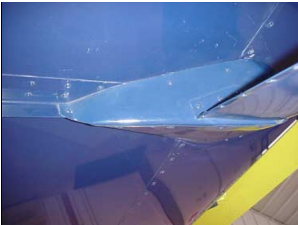
L angle in the corner of the bottom wing skin riveted along the bottom edge of the Top Fairing.
