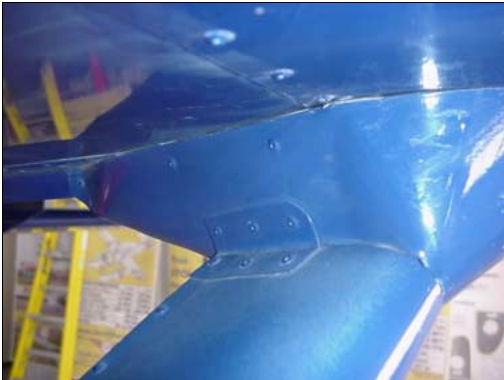
Short piece of L angle between the O/B fairing and the top fairing.
