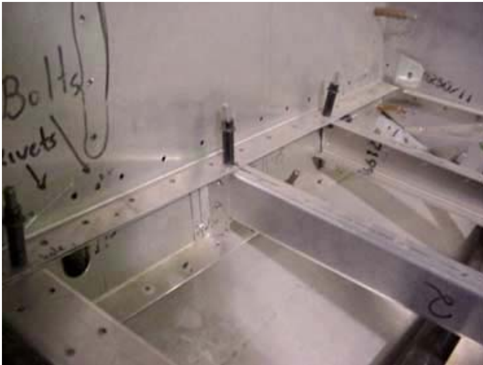
L angle riveted to the side of the stiffener and inside the Rear channel
