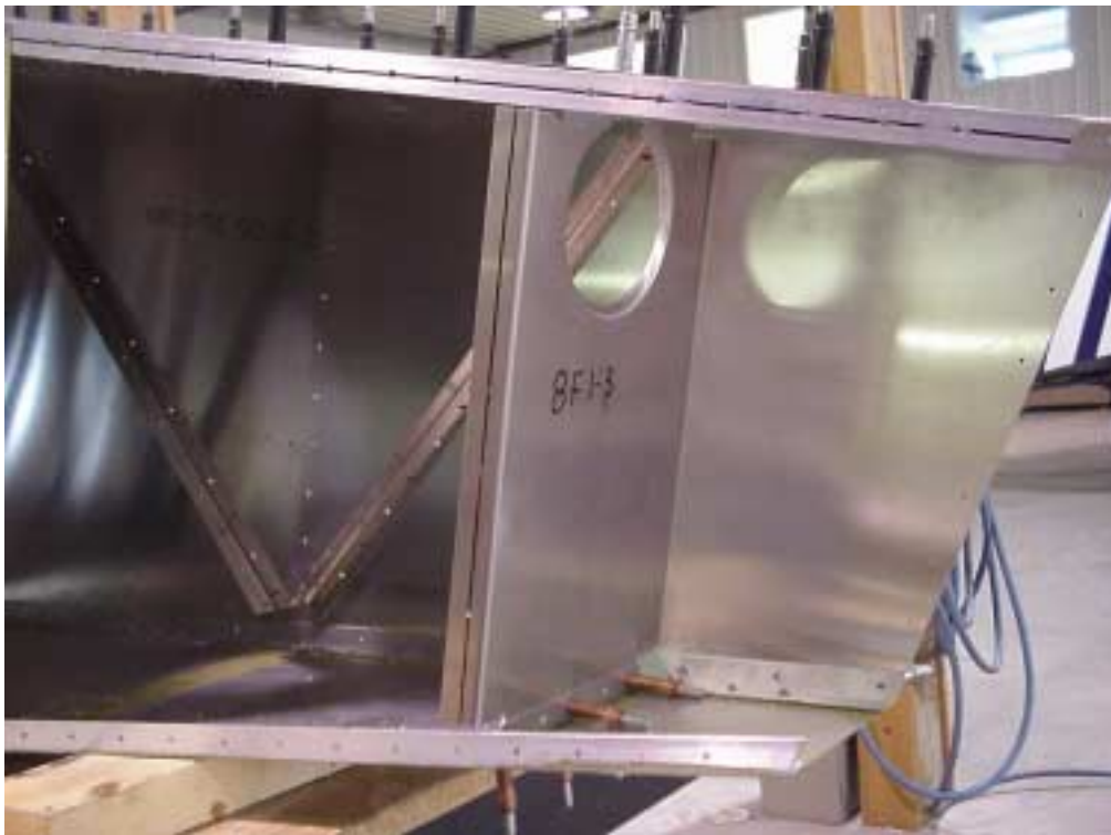
Install an L angle at the bottom of the H.T. Frames and the bottom skin.
