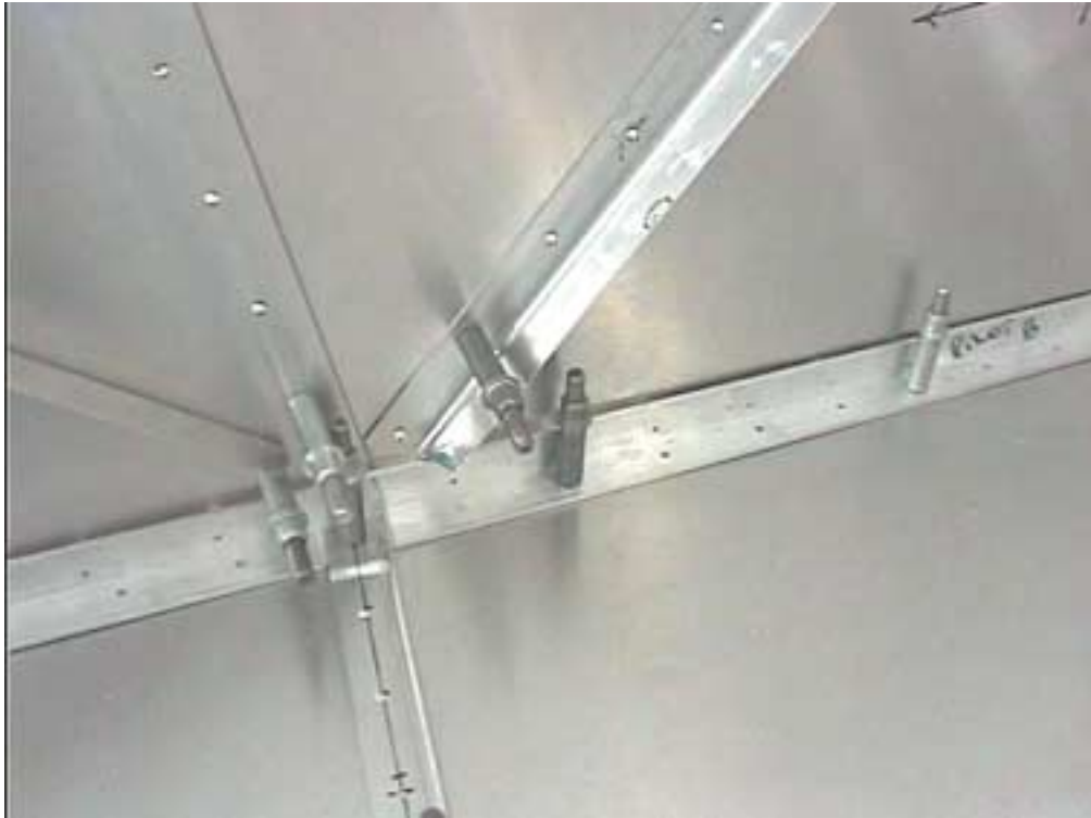
Corner detail of longerons to bottom and side skins.
