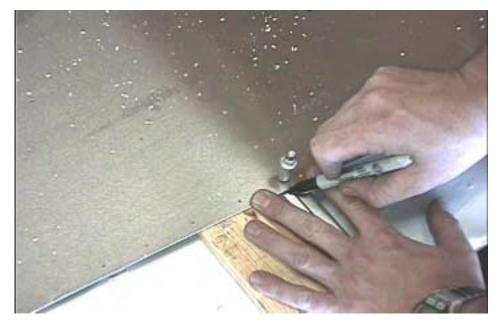
Position the L angles under the skin, drill & cleco. Trace the sides of the skin to mark the length of the L angles. Remove and trim.
