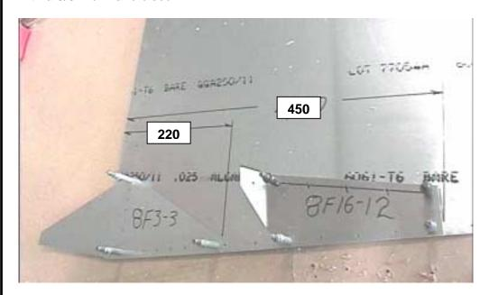
Locate gusset 8F3-3 as shown in the photo. Drill the rivet holes with a 3/32" drill. Do not rivet.
