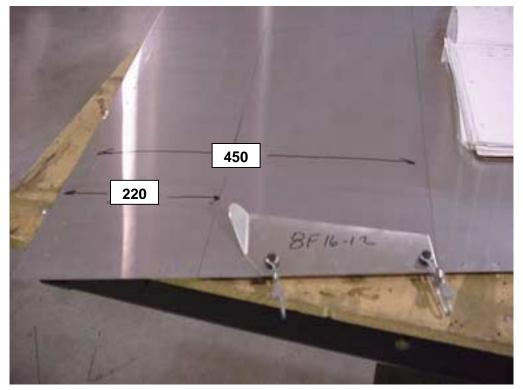
Locate the seat belt attachment bracket 8F16-12 as shown. Drill all the holes with a 3/32" drill and cleco.
