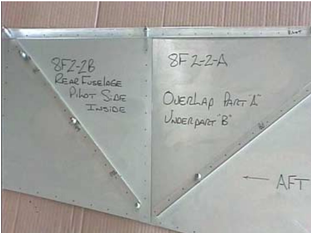
Detail of the diagonal L angles forward and aft of the side skin overlap.
