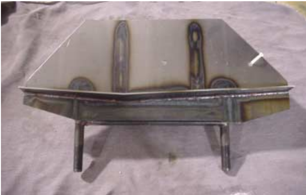
The flange on the I/B side fits underneath the cabin frame.
