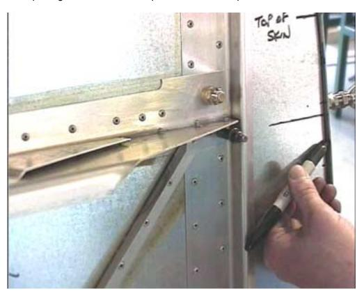
Do not trim the skins any longer than 3mm past the firewall as the increased length will make forming the bend later very difficult.
