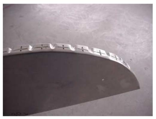
Layout the rivet pitch, locate the rivets between the crimps on the firewall and for the instrument panel.
