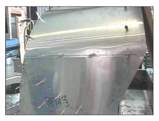
Skin over the instrument panel and the firewall. The bottom edge is trimmed after the skin is drilled.
