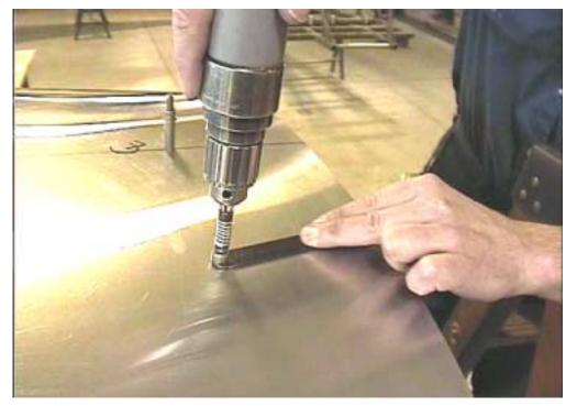
Work one side at a time: Either use a hole finder and drill down from the top, or tape the bottom edge to the side skin, and drill up through the pilot holes in the flange.
