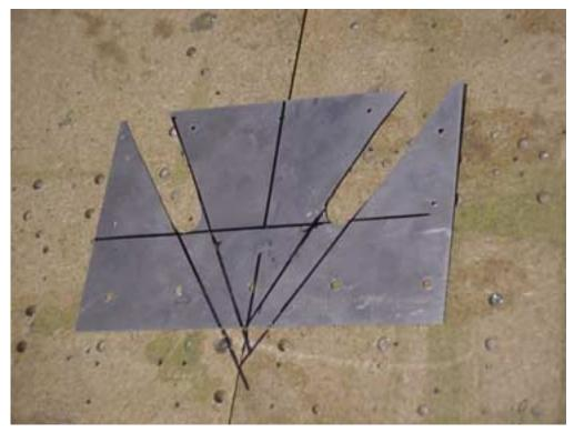
Size: 190x120mm Cutout to make room for the front tube welded on the cabin frame. Use the cutout on 8F14-9 to layout the cutout on the top skin 8F14-5
