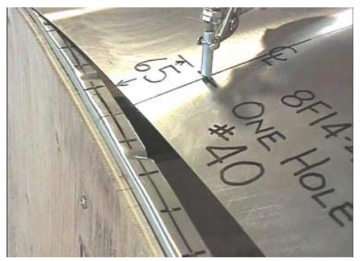
Drill pilot holes on the aircraft centerline through the rivet line in the instrument panel and the firewall
