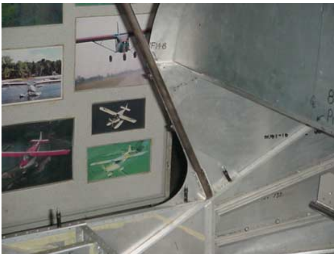
Gussets at the end of the side tube on the cabin frame
