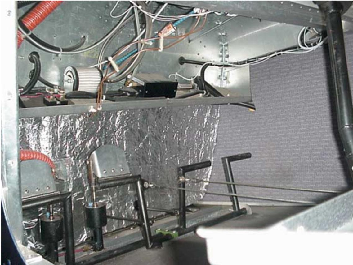
8F7-7 used as a convenient mounting tray for accessories: filter for vacuum pump, shunt, and transponder encoder
