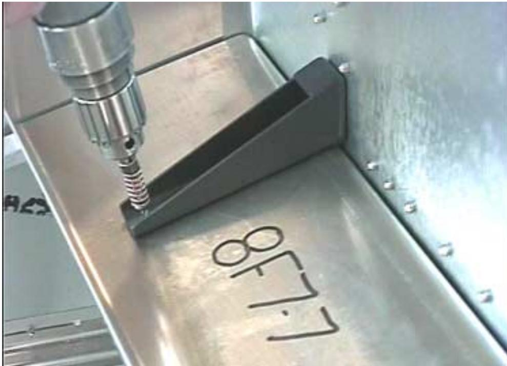
Position the Upper Horizontal Z rear 8F7-7 on top of the “front cabin side Longerons” with the 30mm flange pointing down against the firewall.
