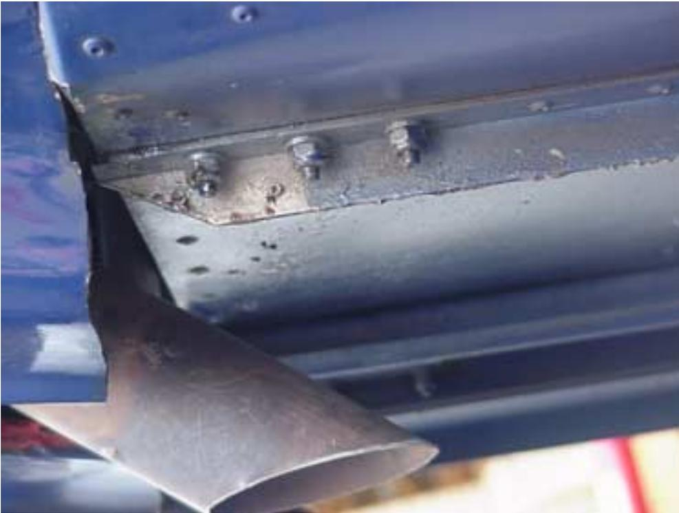
Bolts Lower Engine Mount brackets 8F7-12 and the Lower Longerons 8F10-3
