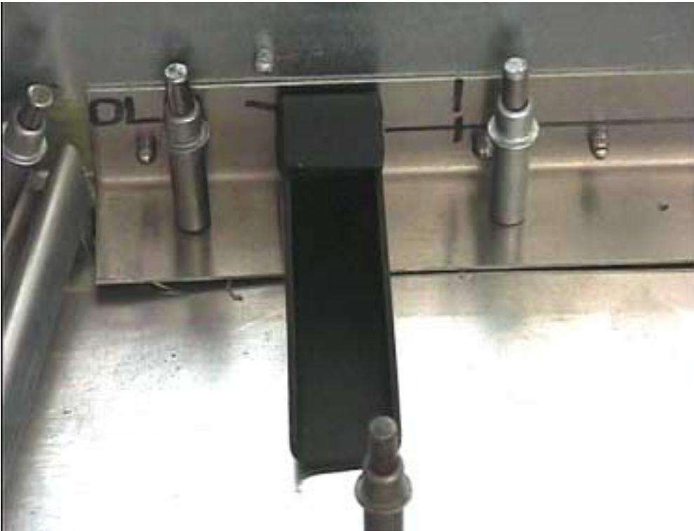
The mounts are positioned by placing the vertical centerline behind the 1/8" engine mount location hole on the firewall.
