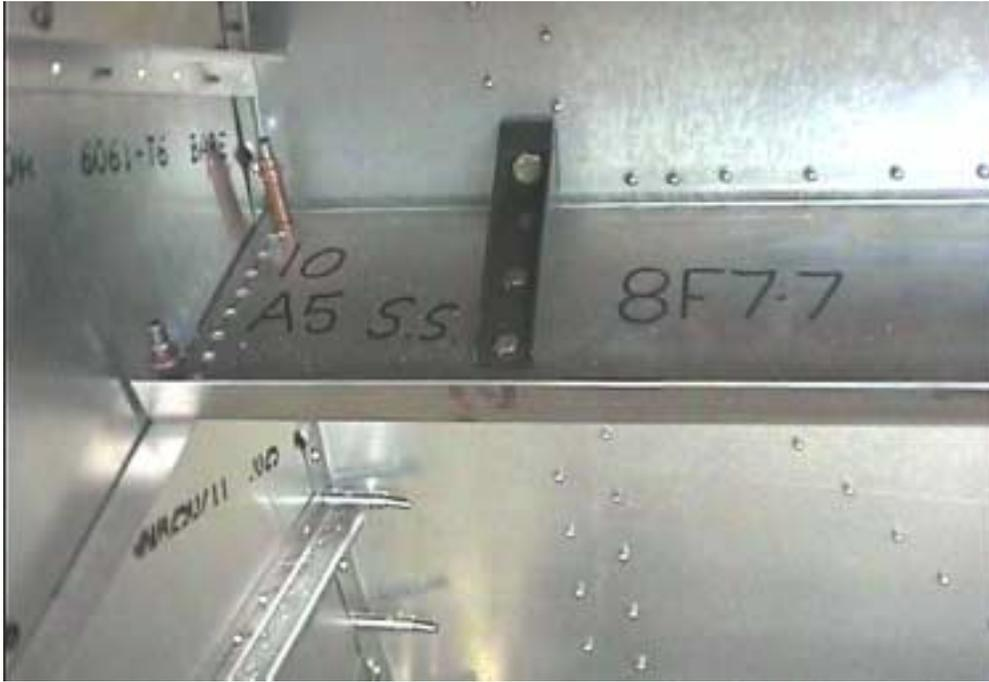
Clamp the cabin side extrusions to the underside of 8F7-7 Check that the Longerons made contact with the side skin
