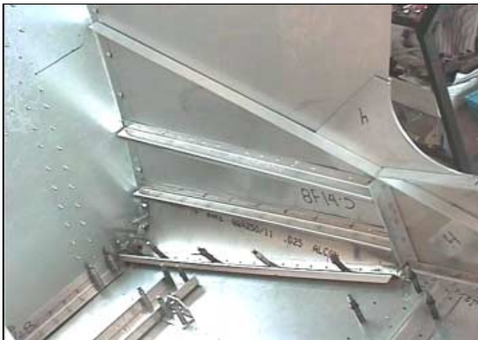
Photo of right inside- Front Side Skin fits between the front of the cabin side assembly and firewall
