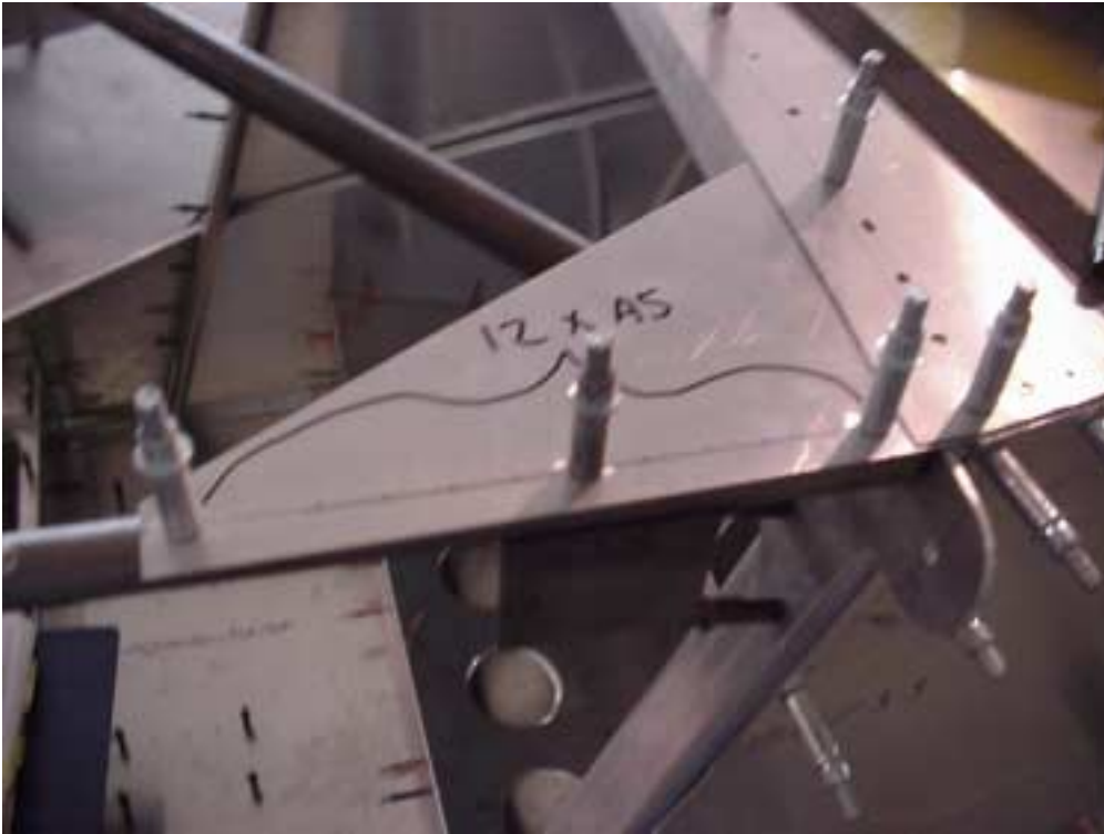
Rivets in the top tubes of the cabin frame and Top Longeron Gusset 8F3-3.
