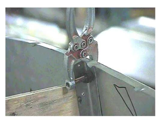
A short piece of std "L" can be used to clamp the jig to the firewall.
