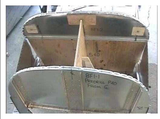
Screw the Instrument panel template A to the Firewall template C, add the template support B to the side of C.
