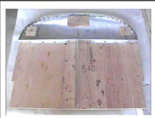
Instrument panel bolted to the <u>backside</u> of the template.
