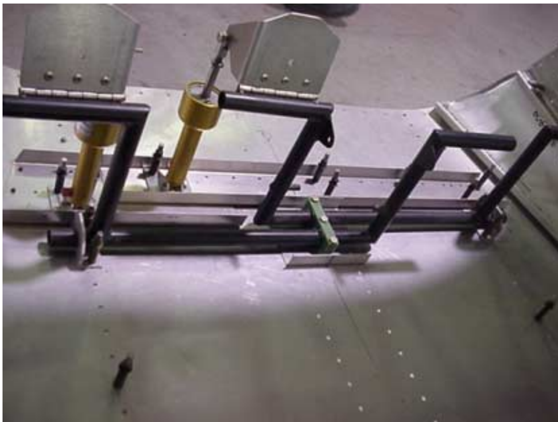
Left and right BRAKE PEDALS 8C4-7: The bend on the right pedals is O/B; the bend on the left pedal is I/B.
