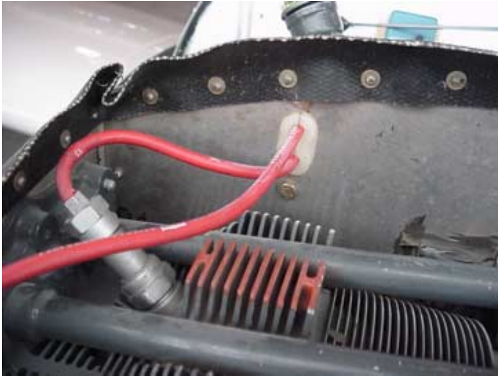
The Wire Seal and the Nylon self-locking nut is on the backside of the baffle.
