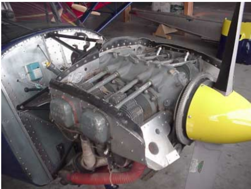
STOL CH 801 Lycoming O-360 engine with baffles
