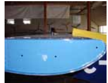
The skin overhang approximately 20mm past the end of the ribs.
