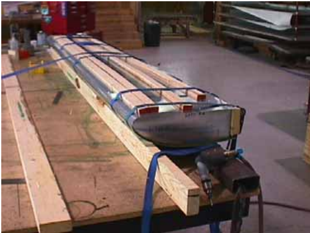
The 1x2 boards underneath the straps help apply a more even pressure on the skin.
