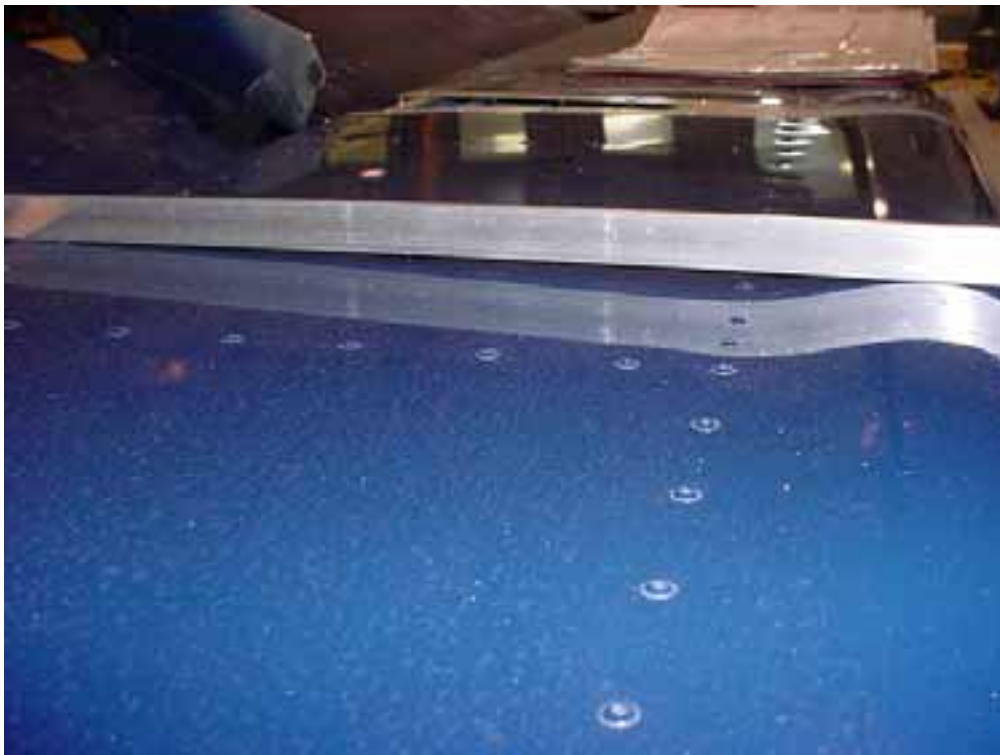
A small gap between the straight edge and the front spar rivet line is acceptable.
