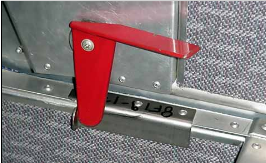
The closed door latch system with the strike plate 8F19-12
