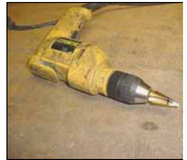
Unibit in electric drill
