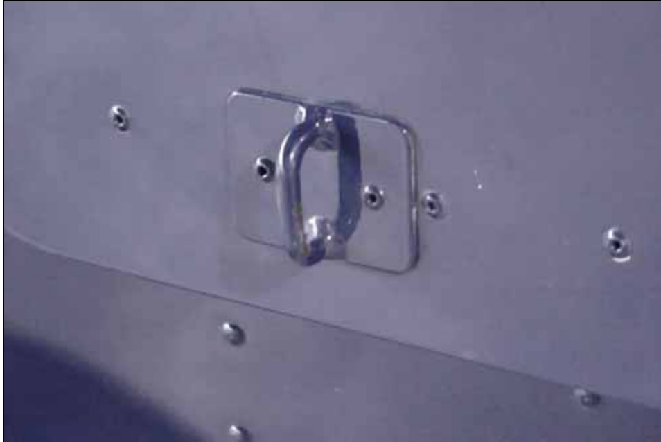
8F19-21 DOOR RETAINER (welded assembly)
