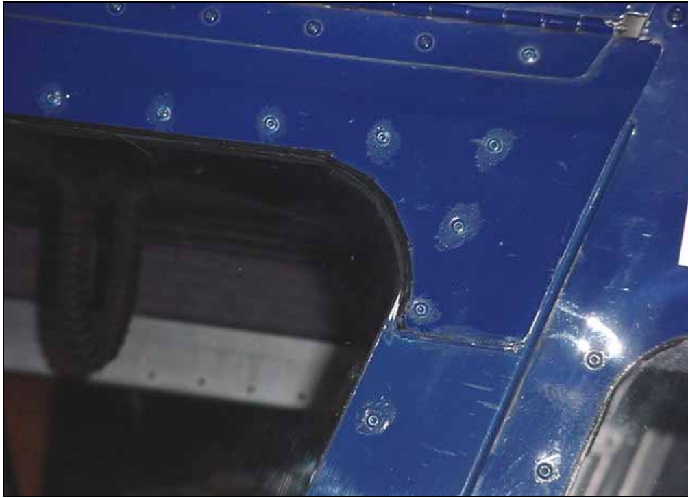
Detail of top aft corner of LEFT door. 8F19-7 and 8F22-9 overlap the fuselage skin approximately on 20mm
