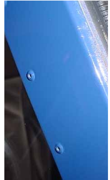
Front right detail, in the closed position the front trim covers up the screws through the windshield.
