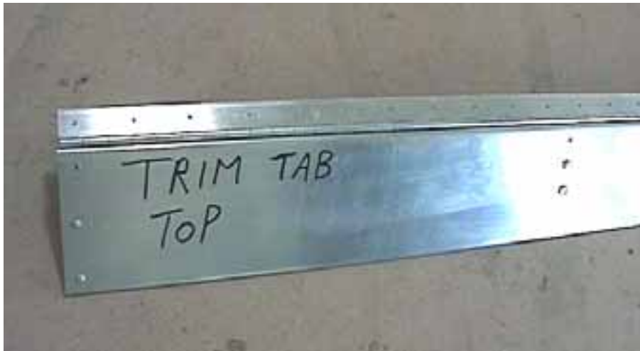
A3 PITCH 40 (through bottom skin, hinge and trim tab flange)
