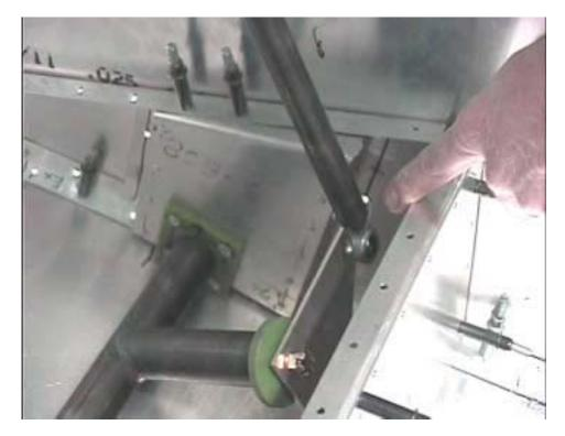
The vertical control rods 8C9-2 will be installed after the wings have been mounted
