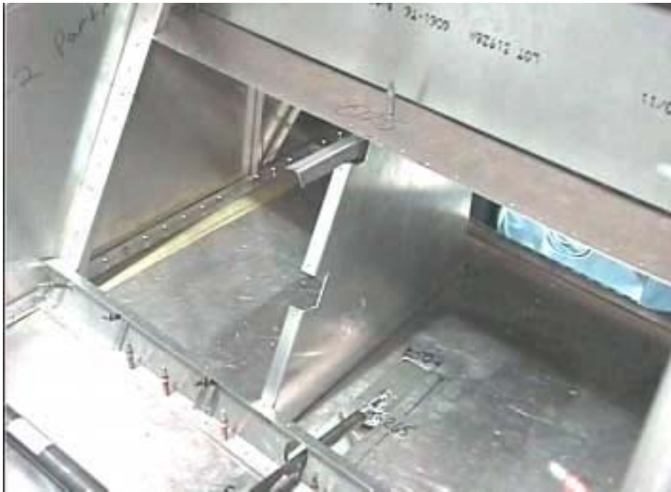
Cutout in the rear fuselage bottom skin to make room for the aft end of the Elevator control Rod 8C8-16
