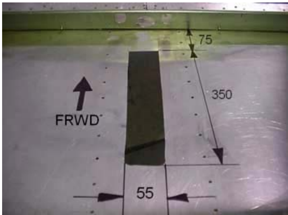
Cutout in the rear fuselage bottom skin to make room for the aft end of the Elevator control Rod 8C8-16
