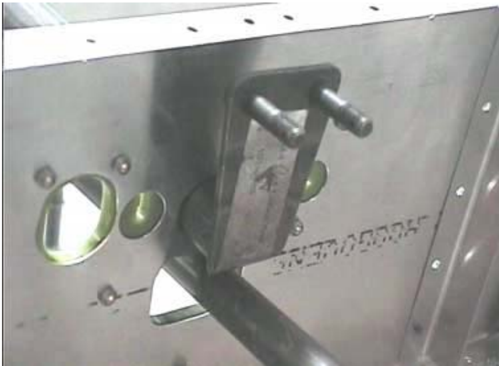
Orientation of 8C8-3 The bolts are towards the top.
