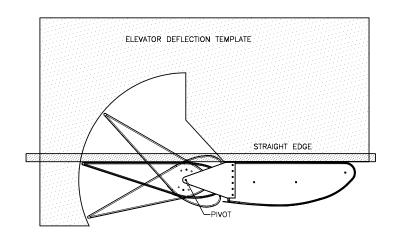
NEUTRAL: TOP SURFACE OF ELEVATOR IS EVEN WITH TOP OF STABILIZER.
