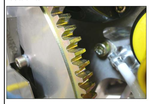
Ground cable is attached to engine mount plate with an M6 bolt. It is located behind the flywheel.
