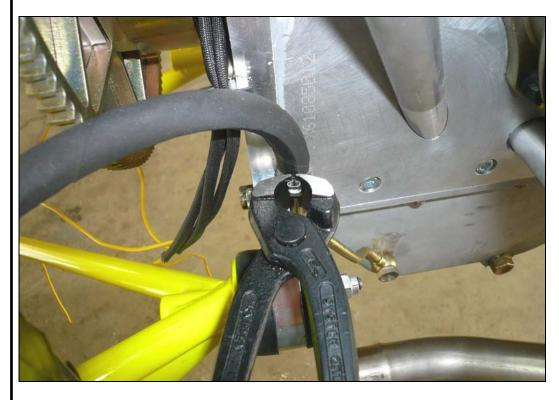
Use Oetiker Crimping Pliers to tighten the Hose Clamps.
