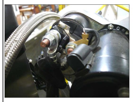
Secure the Pos. Wire to the Starter Soleniod with a self locking nut.
