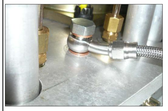
Oil pressure is measured in the main oil gallery on the left side of the engine casing. Do not over tighten the banjo bolt in to the engine case. Torque to 25Nm.
