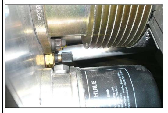
This picture shows the installed Oil Temp Sensor and Oil Filter Sandwich Plate with Thermostat.
