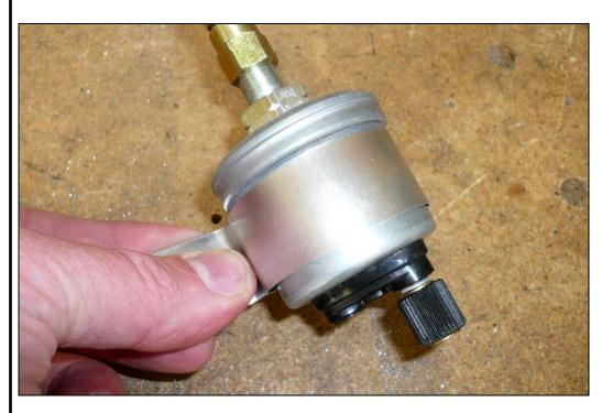
Use a piece of extra material to make a strap to hold the oil pressure sending unit to the ULICP ignition coil mounting plate (see below). Oil pressure sending unit may very in size. Oil Pressure unit needs to be compatible to your instruments.
