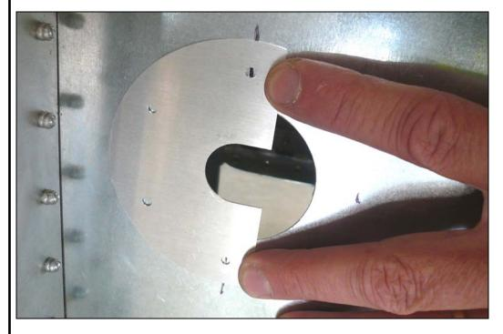
Measure up 320mm from the bottom of the firewall and 120mm from the center to locate firewall grommet. Drill a 2" hole with a hole saw so the ECU plug can go thru the firewall.
