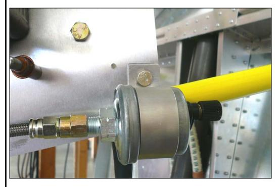
Mount the oil pressure unit on the Coil Mounting Plate with the bolt to the adel clamp. This unit the case is the ground and the post goes to the instrument panel.
