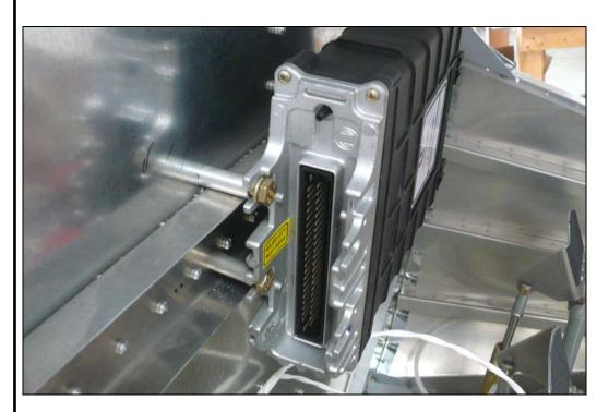
Mount the ECU (Engine Control Unit) on the inside of the firewall using the ECU spacers with AN4-14A bolts. For ECU Positioning and wiring see ULPOWER Installation Manual.
