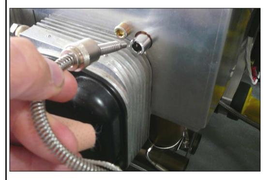
All four cylinders should have a CHT probe Each cylinder head has a pre-drilled hole close to the exhaust port to monitor CHT (see avionics installation manual).
