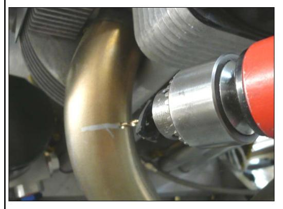
Installation of the EGT Probes: Measure down 3 inch from the beginning of the exhaust piping. Drill with a number 20 drill bit.
