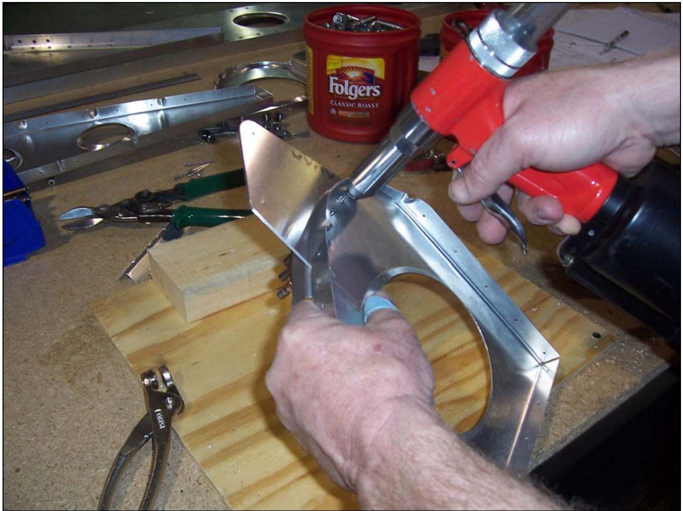
Deburr and rivet the L angle and Slat Support to the Nose Rib with A4 rivets.
