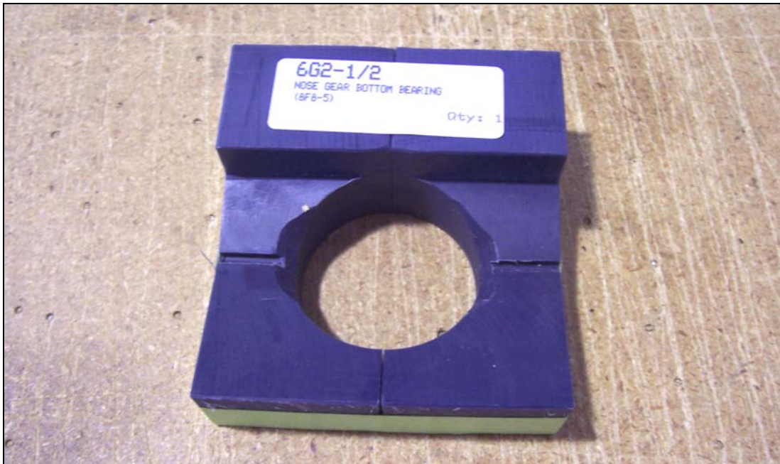
P/N: 75L1-7 Nose Gear Bottom Bearing
