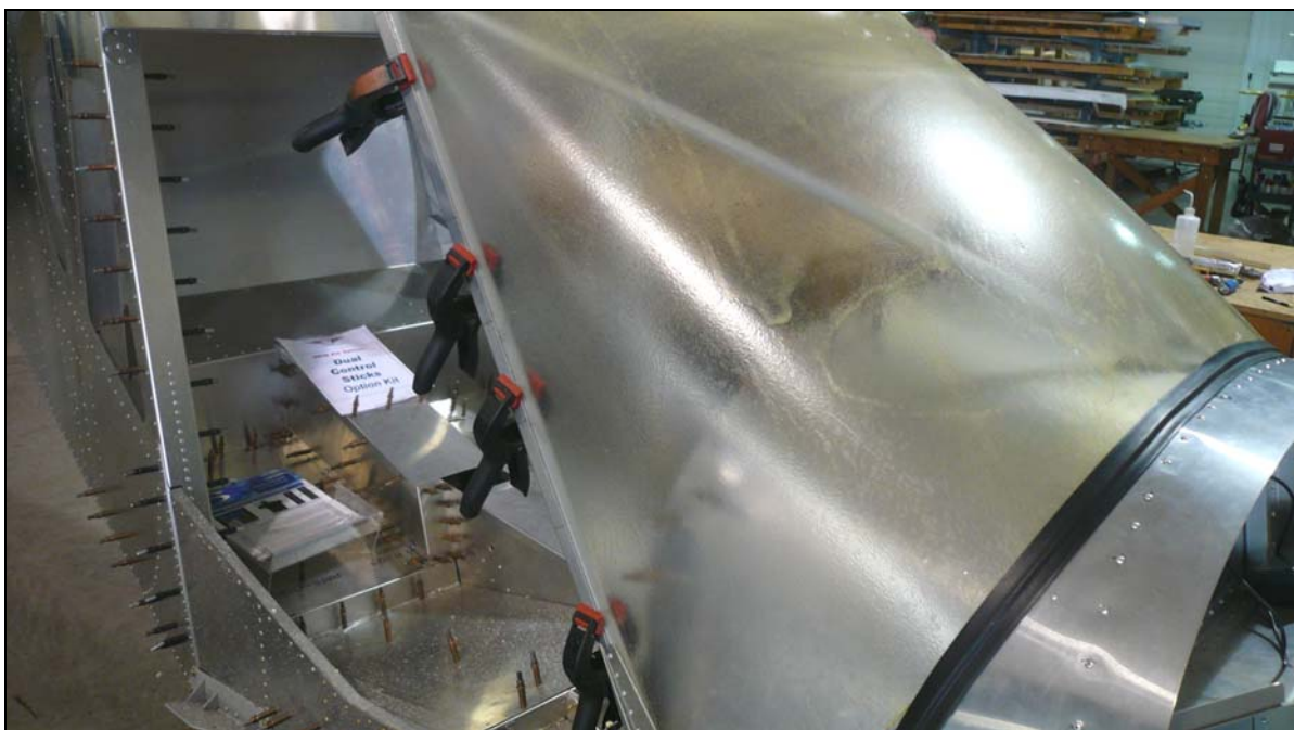
Use the 60 degree special drill bit for Acrylic to drill the screw locations on the Side Trim into the Windshield and Cabin Frame and Cleco. Expand the holes to 1/4" in the Windshield only using 60 degree special drill bits and Cleco.
