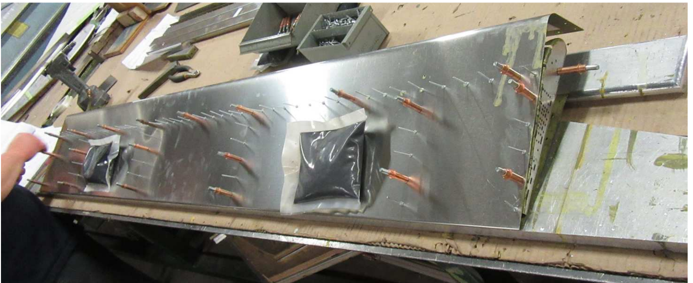
Drill all the holes and rivet.
