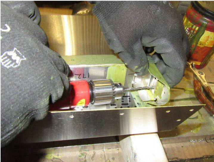
Back drill into the full rib and cleco
