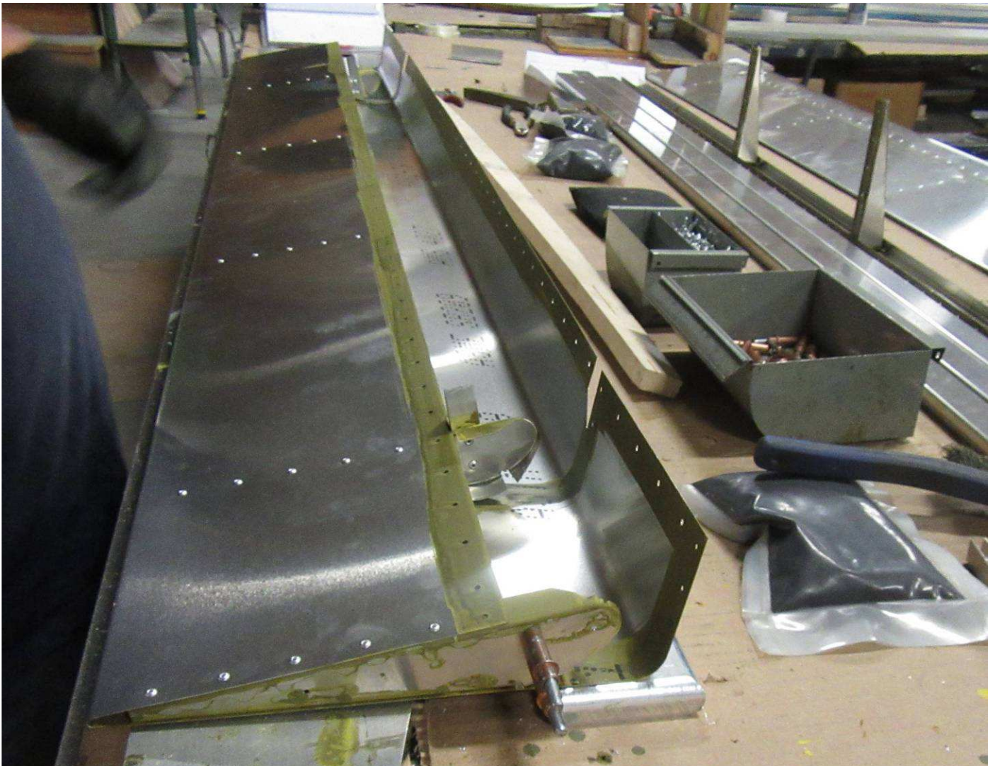
Back drill into the full rib and cleco
