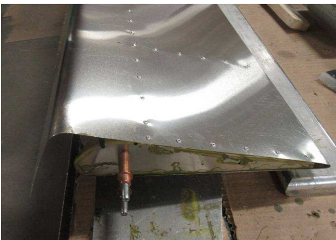
Rivet the top side: rear ribs and spar.
