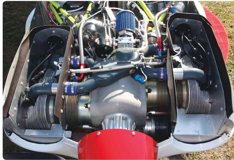
*A direct drive, thoroughly traditional engine, the 130-hp ULPower UL350iS incorporates the latest in electronic ignition and FADEC control.*
