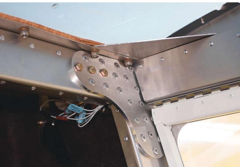
*The CruZer uses aircraft-grade pulled rivets throughout.*
