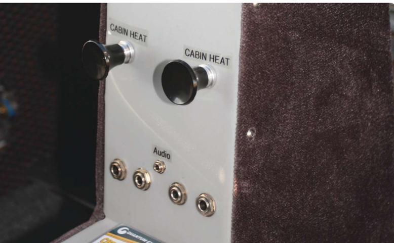
*The console mounts pilot/co-pilot heater controls.*
