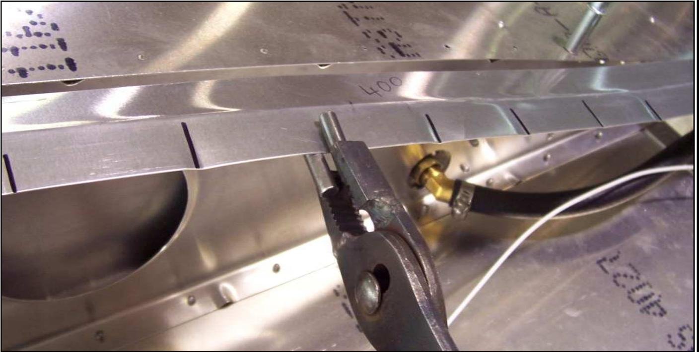
Put crimps on the marks in the flange of the Wing Root Angle to match the curvature of the Ribs.
