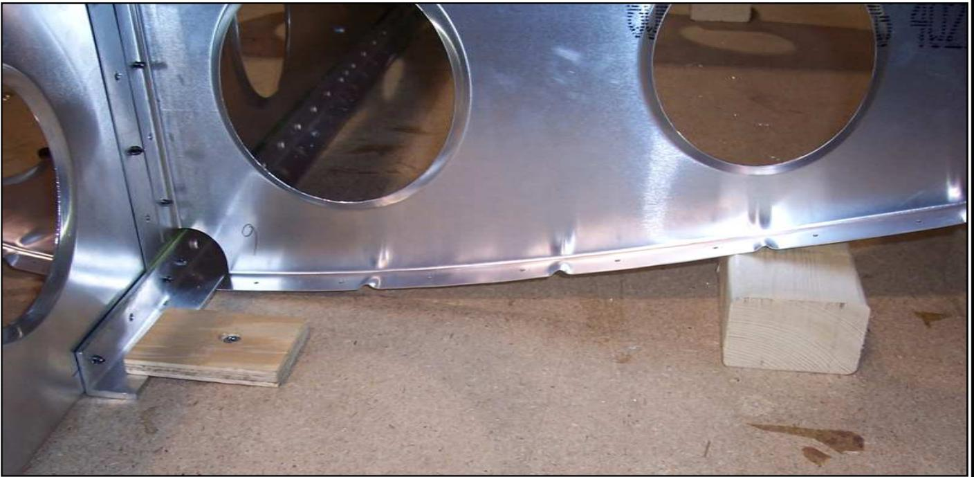
Screw pieces of plywood to the workbench to secure the Wing Skeleton. Slide pieces of 2"x4" under the Rear Ribs to rotate the Spar till it is vertical.
