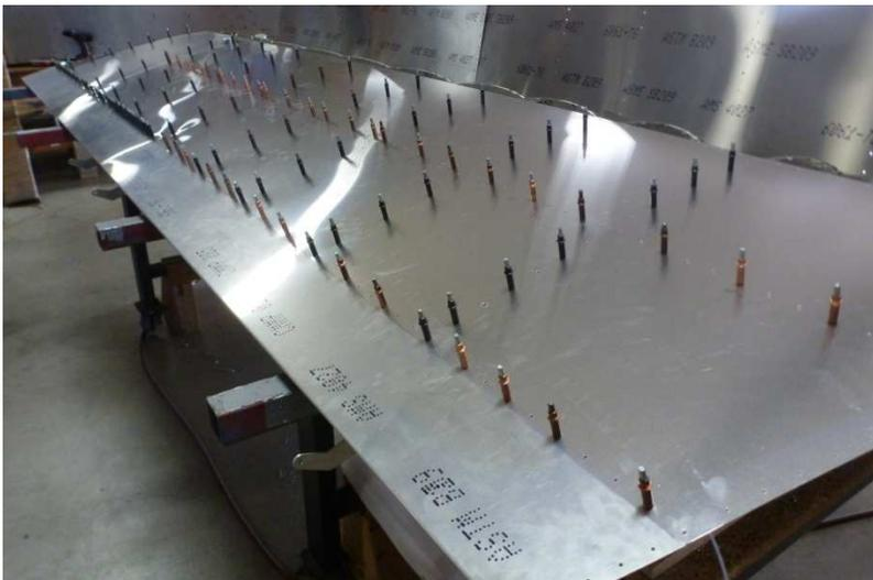
Back drill through the Top Skins in the Trailing Edge Skins and Rear Channels with a #40 drill bit when the Trailing Edge is set at the correct distance. With a #30 drill, expand the holes. Use a #20 drill bit to expand the holes on the inboard end of the wing: from the root to the rear channel splice, See drawing C75-WA-1 and C75-WA-2 for details.
