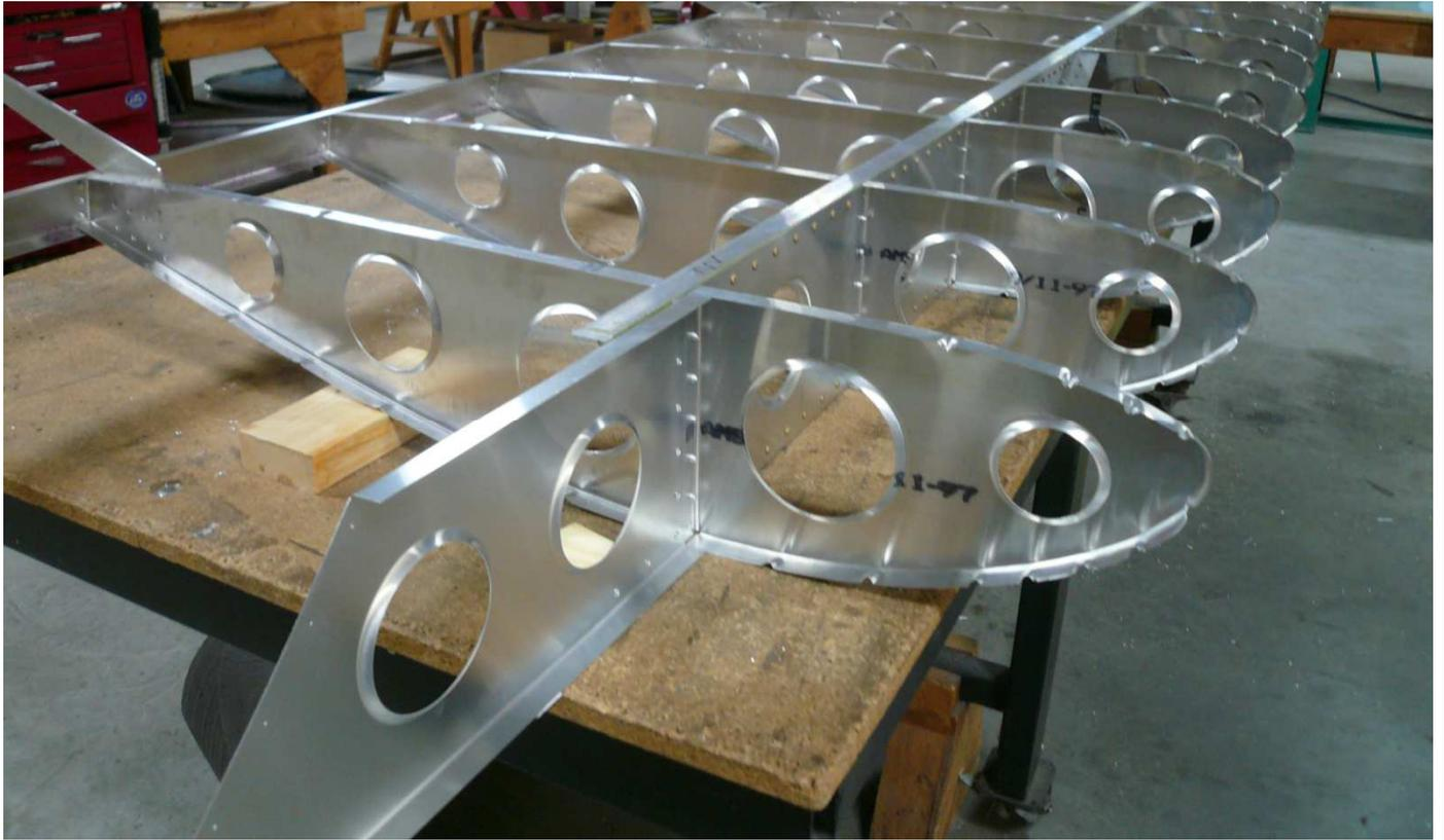
**Check:** Check that the Spar is vertical at several locations down the length of the Spar. This will prevent twist being built into the Wing.
