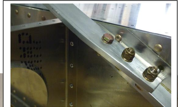
**Note:** The first bolt must be inserted from the bottom with the nut towards the inside of the wing to clear the Nose Skin.
