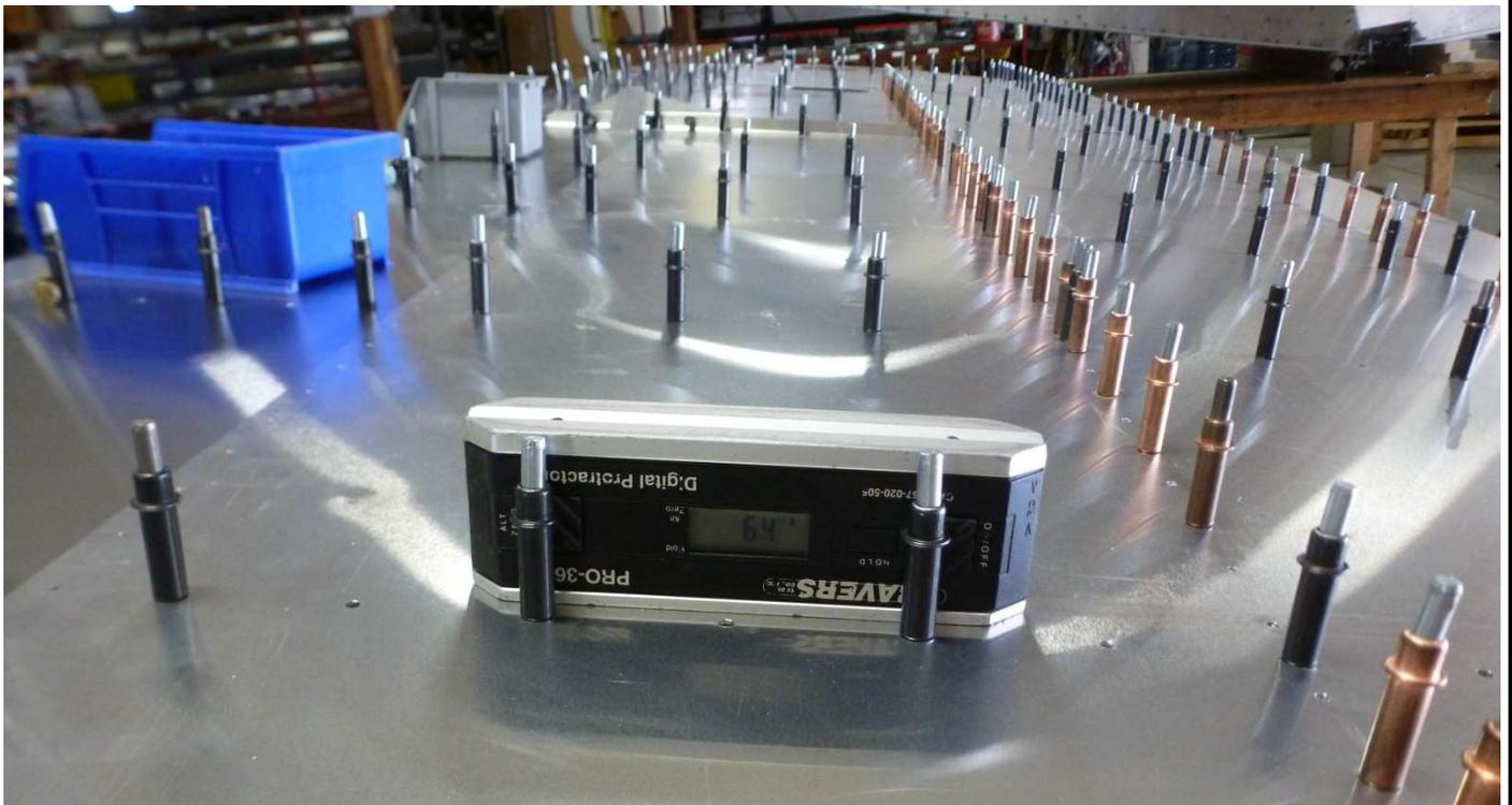
**Note:** It is a good idea to check that the Spar is still vertical before reassembling the Skins and riveting. Even after the holes are drilled there is enough play in the Clecos to introduce twist if the Spar isn't vertical.
