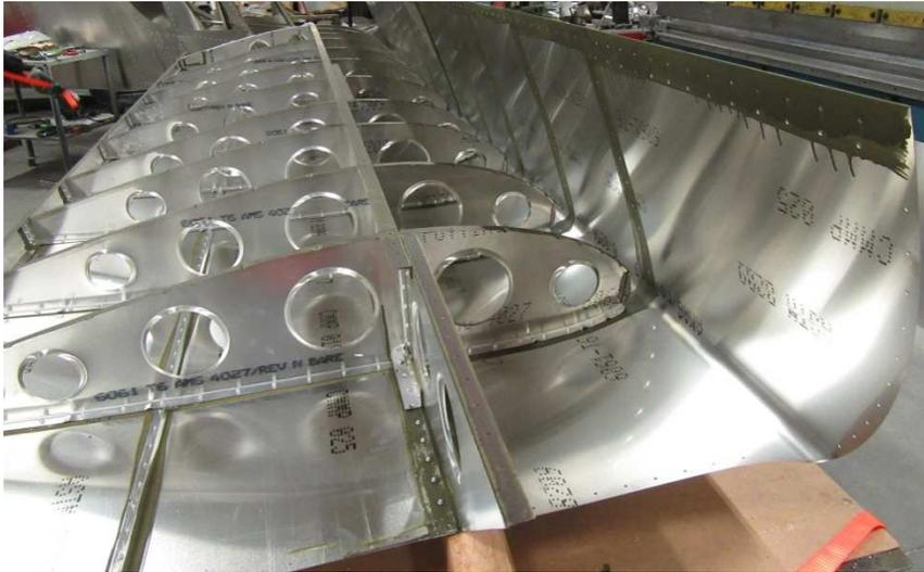
Flip the Wing over and set it on several beams. 2"x2" steel beams are used in the photo above but any rectangular or square beam 2" tall will work to lift the wing above the workbench. It is a good idea to place a piece of plywood under the Rear Channels on the beams to prevent the Wing from rocking.
