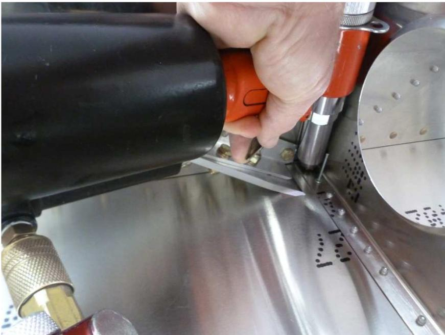
With the front upper strut fitting bolted in place, the rivets are pulled from the top side of the wing. (After the wing is turned over).
