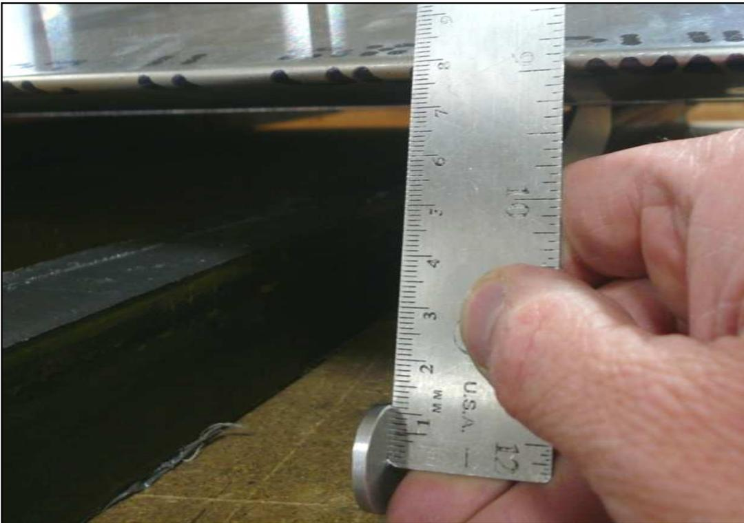
Set the Trailing Edge Skin height at 80mm from the hole in the Flaperon Arm to the center of the radius of the Trail Edge Skins.
