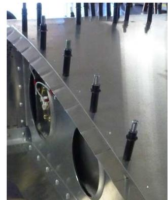
Crimp the L angle to match the angle of the Wing Root Angle and the Root Nose Rib. Be sure the Crimps are between rivets locations.
