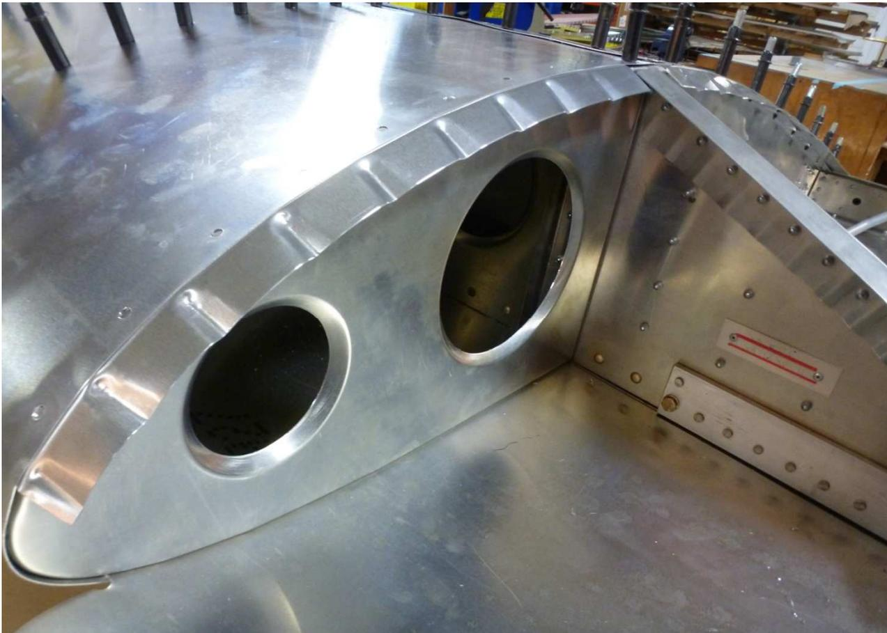
Slide the Wing Root Angle under the Nose Skin and I/B Top Skin. Back drill with a #30 drill bit through the Nose Skin and I/B Top Skin into the Wing Root Angle.
