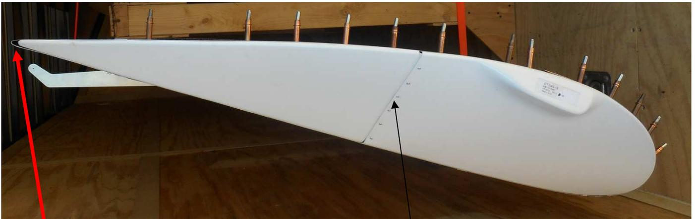
A small gap at the trailing edge is normal.
