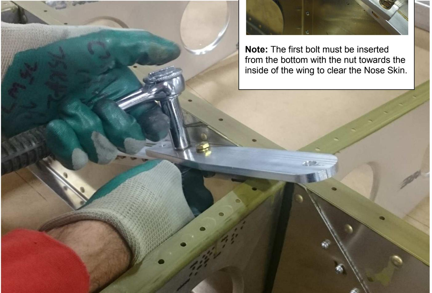
Bolt the Front Upper Strut Fitting to the Strut Angle on the Spar with 3 AN4 bolts.
