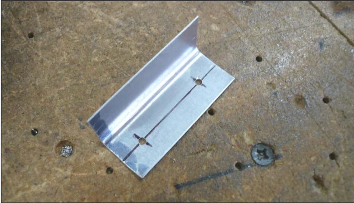
Cut two L Angles 50mm long. Draw a center line on one flange of the L Angle. Mark rivet locations 10mm from each end of the L Angle. Use a #40 drill bit to drill the rivet locations.
