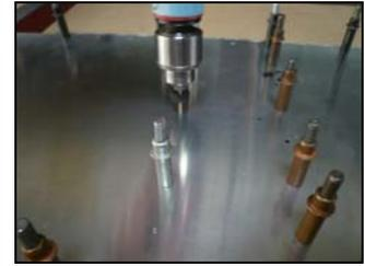
Back drilling the "L" Angle next the Trim Motor.
