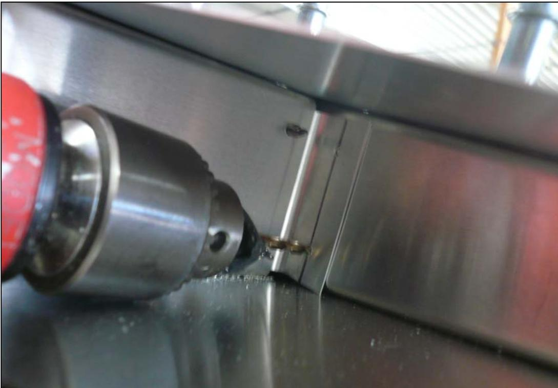
With the top Skin clecoed to the Ribs and Channels, back drill through the holes in the L Angle into the Inboard Ribs with a #30 drill bit and cleco. Expand the holes with a #20 drill bit and cleco.
