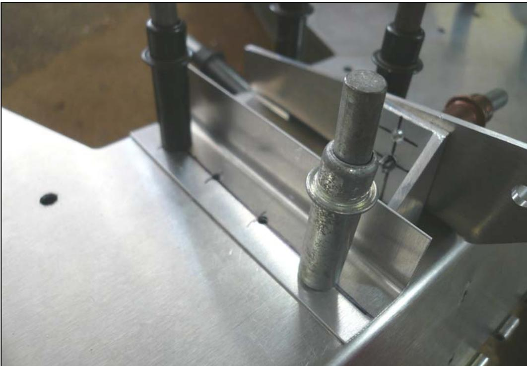
The 82mm long L Angle is installed on the bottom of the Elevator. Cleco the aft hole in the L Angle to the Elevator and Rear Channel. Back drill through the L Angle into the Elevator and cleco. Expand the holes with a #20 drill bit and cleco.
