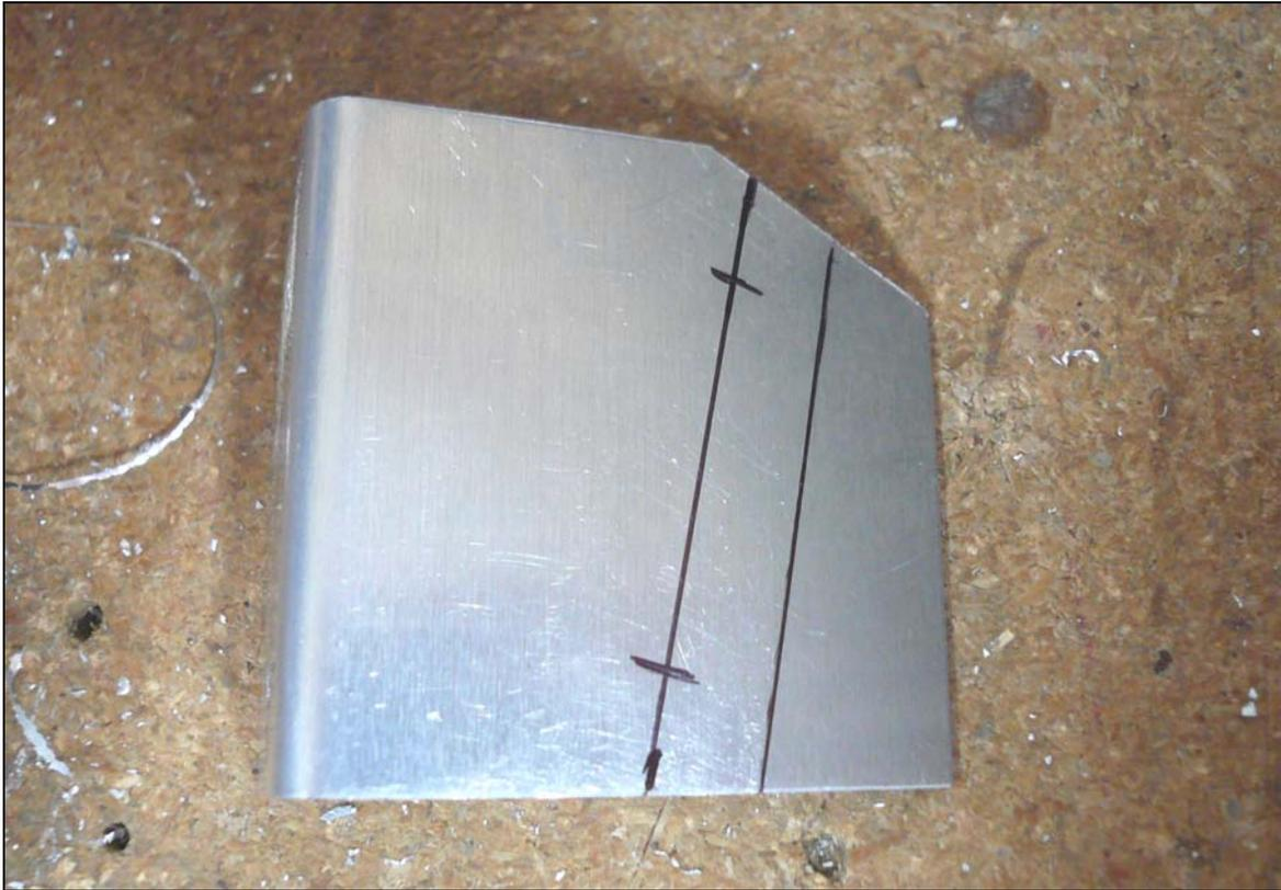
Mark the aft edge of the Doubler on the Angle and remove it from the Elevator. Mark an offset line 10mm from the edge of the Doubler. Mark two rivet locations 10mm from the top and bottom edges of the Angle. Use a #40 drill bit to drill these rivet locations.
