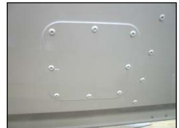
Access Cover can be riveted to the Elevator Skin.
