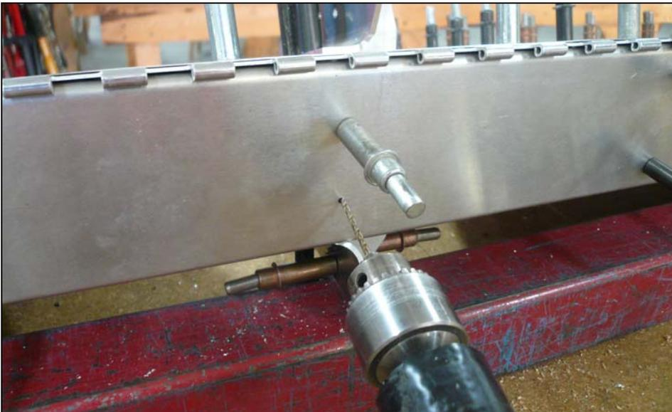
Use a #40 drill bit to back drill through the holes in the Skin into the Angle and cleco. Expand the holes to a #20 and cleco.
