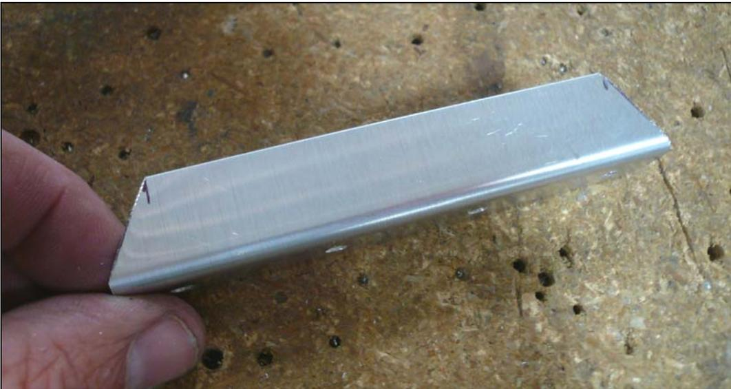
Remove the L Angles from the Elevator. Mark a point 10mm from the end of the undrilled flange. Mark a line from the point to the start of the bend radius. Crop the corners of the L Angles and cleco them on the Elevator.
