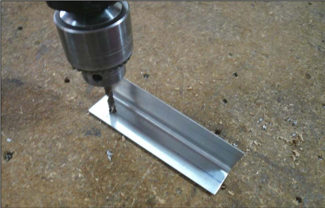
Cut one L Angle 82mm long and another 110mm long. Mark the center line on one flange of each L Angle. Mark the rivet locations 10mm from each end of the L angle. Evenly space 2 additional rivet locations between the end rivet locations. Use a #40 drill bit to drill the rivet locations. Expand the aft most hole with a #20 drill bit.
