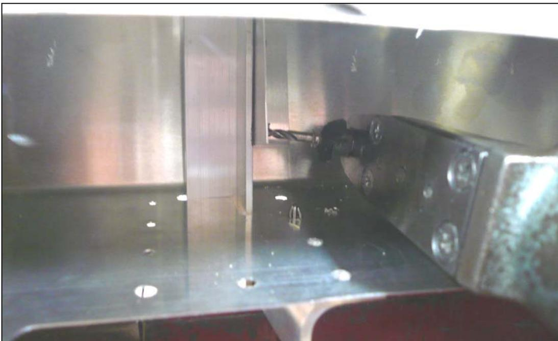
Reinstall the Angle in the Elevator. Use an Angle drill with a #30 drill bit to back drill through the Angle into the Doubler and cleco. Expand the holes with a #20 drill bit and cleco.
