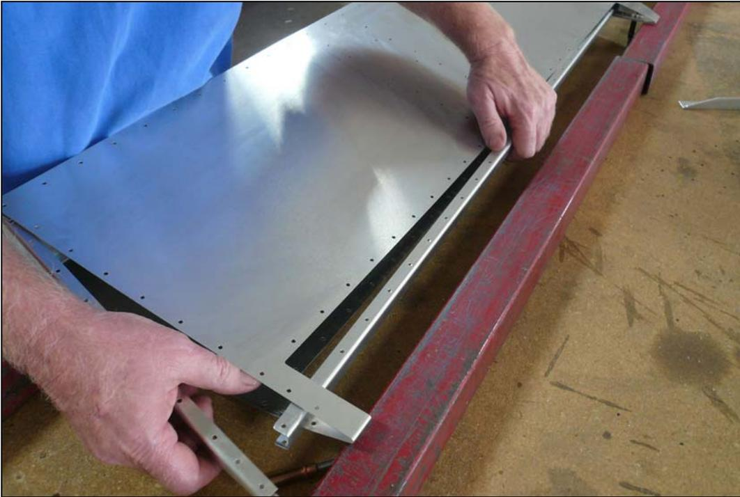
Slide the Cutout Channel into place on the Elevator. It will be helpful to pull the outboard Rib away from the Channel to slide it in place. Cleco the bottom flange of the Channel to the Skin.
