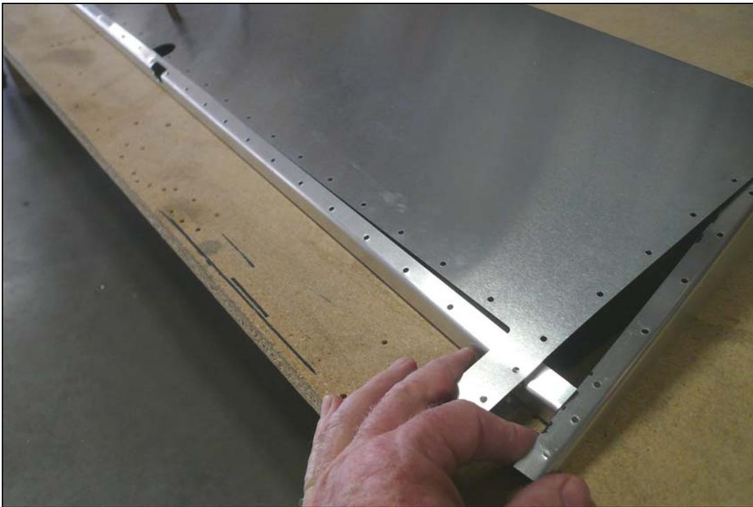
**Orientation:** The cutout in Channel should be installed on the bottom side of the Skin.
