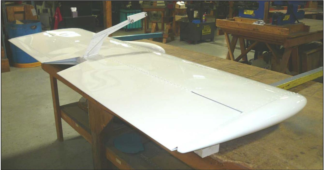
The Elevator and Stabilizer can be mounted together and painted as one unit. After the assembly has been painted the Elevator can be Mass Balanced before mounting on the Fuselage. Balancing the control section will be shown later in the Drawings and Manuals.
