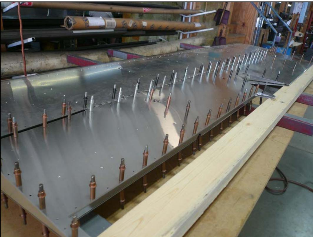
Position the Elevator onto the Stabilizer with the Piano Hinge. Slide the Piano Hinge between the top Skin and flange on the Elevator. Center the Elevator onto the Hinge that is attached to the Stabilizer. Use a #40 drill to back drill through the Skin into the Hinge. Then open up all holes on the Hinge to #30 and then final size to #20 and cleco.
