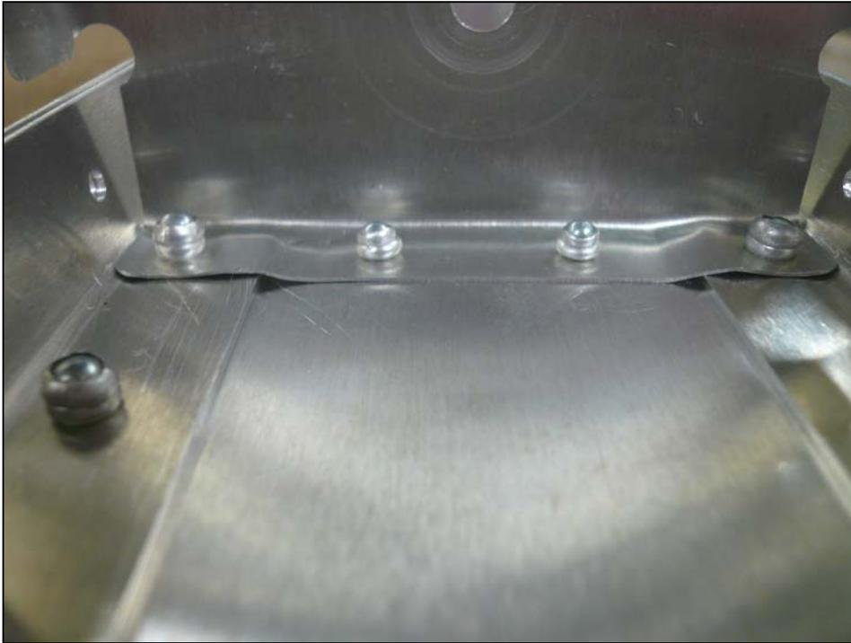
Cleco the Ribs and Rear Spar together. When riveting the Ribs make sure that the flange on the Ribs pull down. Notice the joggle on the Rib.
