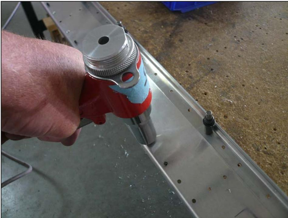
Deburr the lower Doublers and rivet the Rear Spar Bottom Doublers. At this time the top Doublers will not be riveted because the piano hinge will have to be position. Make sure not to rivet the holes where the ribs are located and in the center for the Rear Spar Attachment Bracket.
