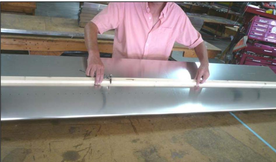
Use a furring strip (1x2 board) to bring the Skin down on the skeleton. Using ratchet straps will also help in holding the Skin down.
