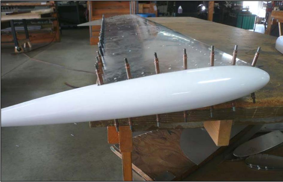
Position the Stabilizer End Cap on each end. Drill and cleco with 1/8 cleco.
