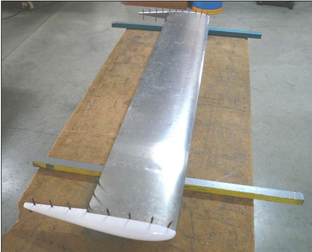
This manual has been prepared for assembly of the Stabilizer using match drilled parts. This photo assembly manual is intended as a supplement to the drawings. If there is any discrepancy between this manual and the drawings, the drawings supersede this manual. For more information on building standards and allowable tolerances see "Construction Standards for Zenair Light Aircraft" available from Zenith Aircraft Co.
