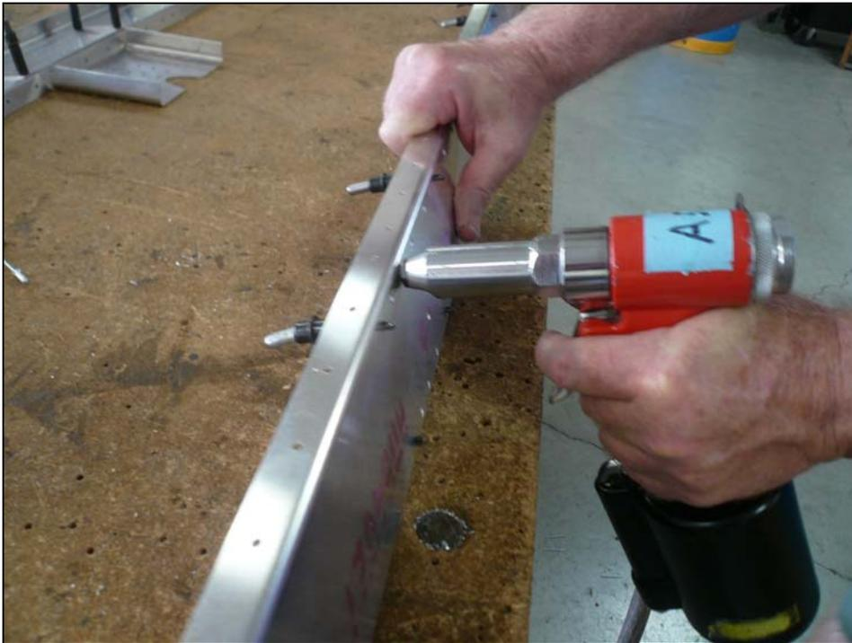
Rivet the Front Spar Cap to the Spar with A5 rivets. Do not rivet in the area for rib location and Front Spar Attachment Brackets.
