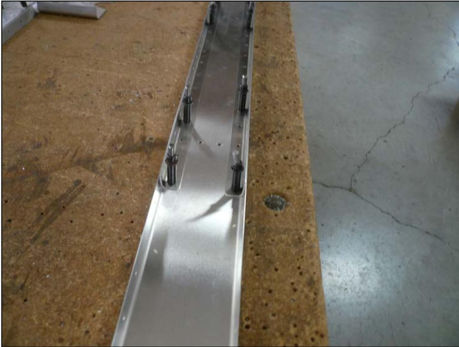
Cleco the Front Spar Cap to the Spar with 5/32 clecos.
