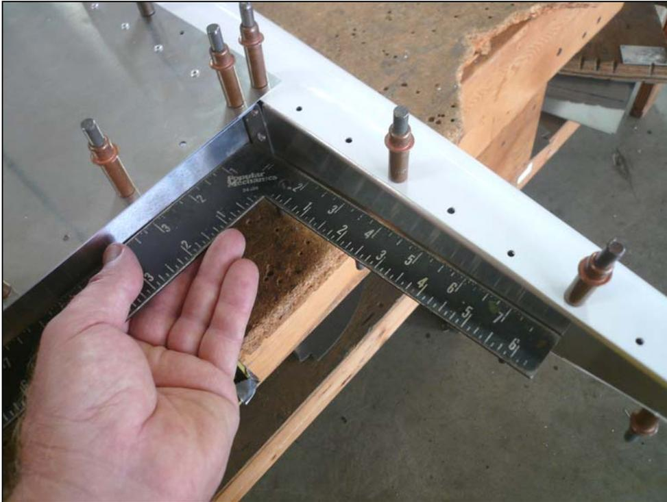
Before drilling check that Rib is square to the Spar. Drill and cleco Cap to the Rib with number 30 drill.
