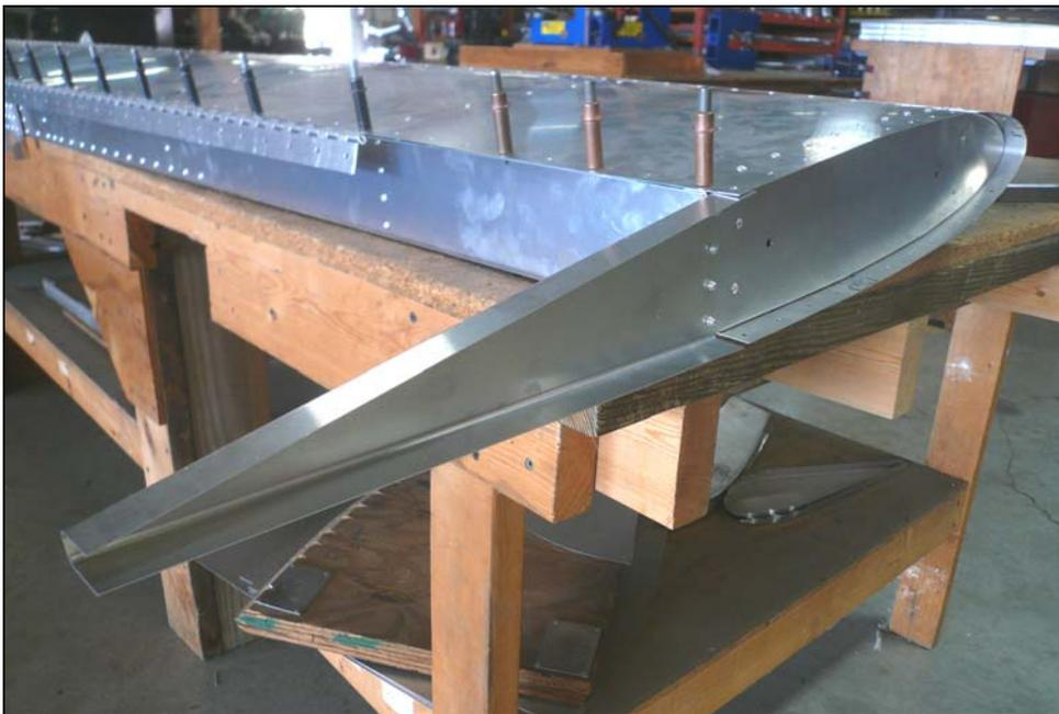
Rivet the Tip Rib using A4 rivets.
