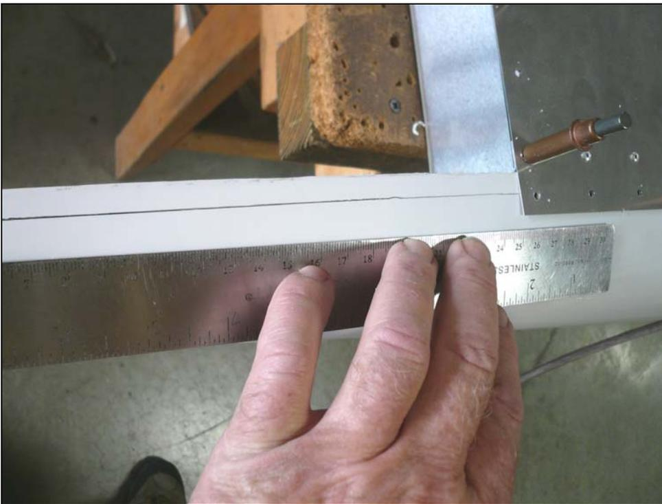
Draw a 10mm rivet line on the Stabilizer End Caps to the aft end. Layout the rivets on the line using pitch 40mm.
