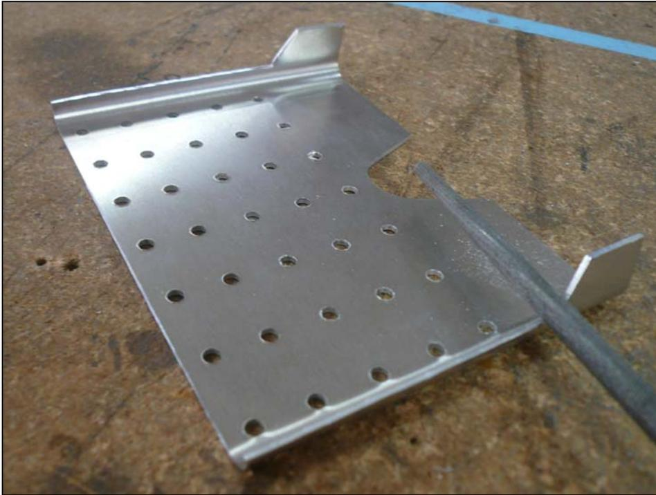
Use a hand file to remove the snip marks and even out the sides. A round file is needed to touch up the corners.
