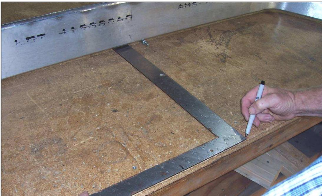
Set a square flush with the edge of the work bench on the center mark. Mark the center line on the aft side on the bottom of the Gear Spring.
