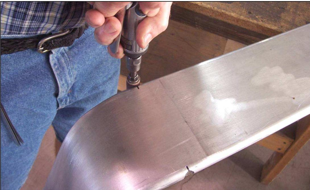
With a die grinder or rotary tool, sand an 1/8" notch into the Gear Spring for each Stud location.
