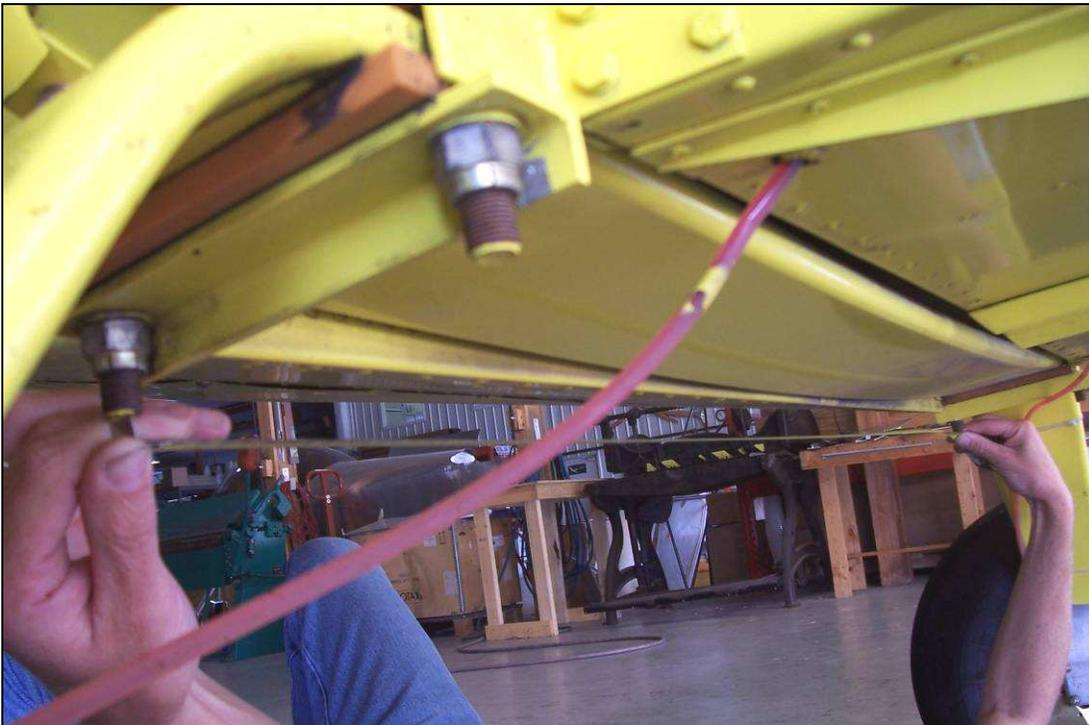
Measure the distance between the studs on the Gear Strut Fittings.
