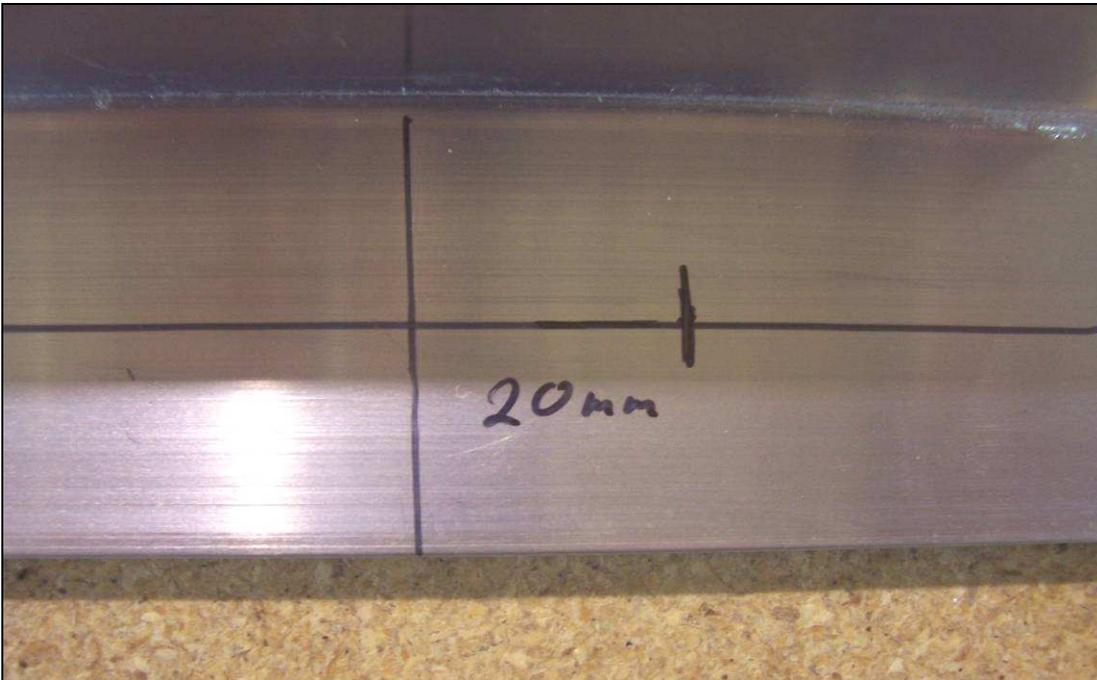
Mark a center line on the flange of the Main Gear Support. Extend the marks for the Stud locations across the center line. Drill the holes out to 1/2" and deburr the holes. Mark a line 20mm from the center of the hole and trim off the excess material from the Main Gear Support.
