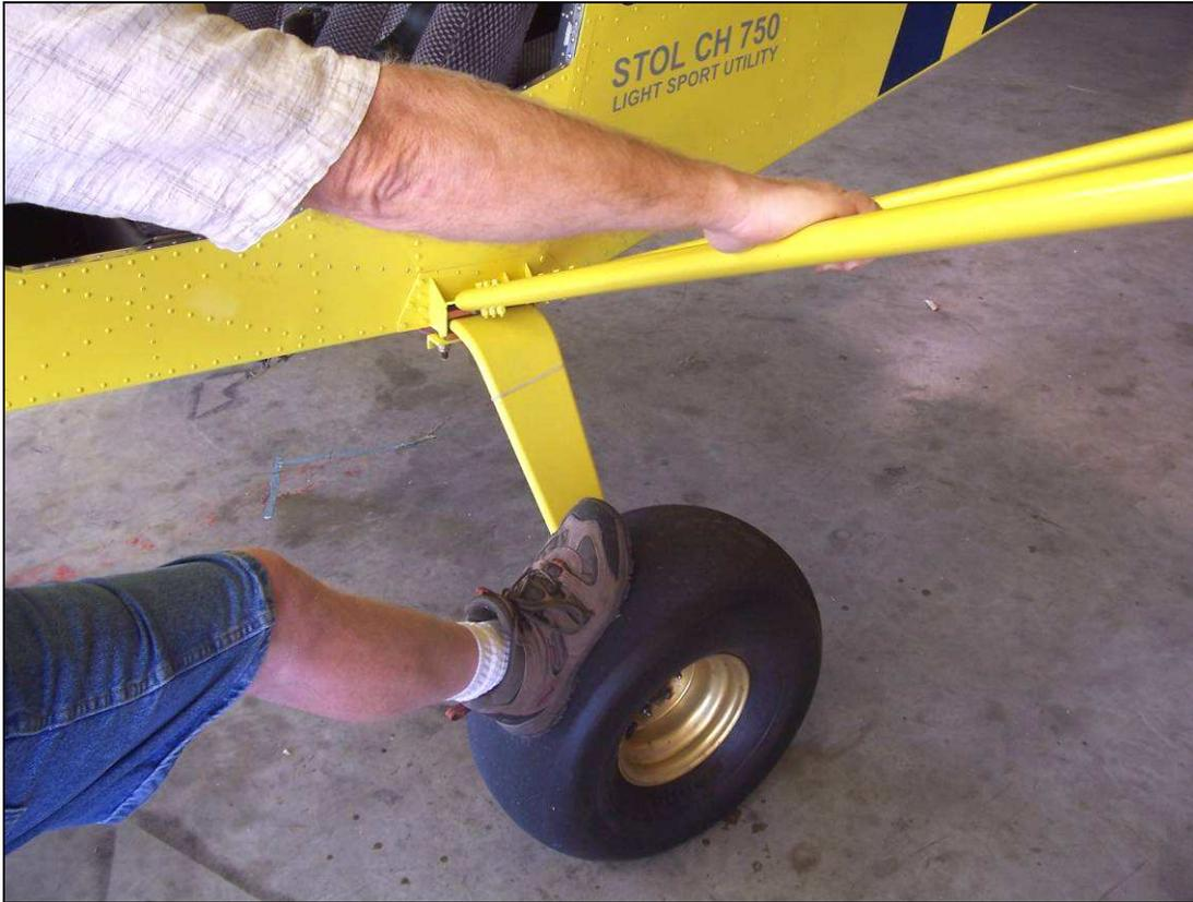
Check to be sure the Gear Spring doesn't rotate after tightening the nuts. If the Gear Spring rotates tighten the nuts further and check again.
