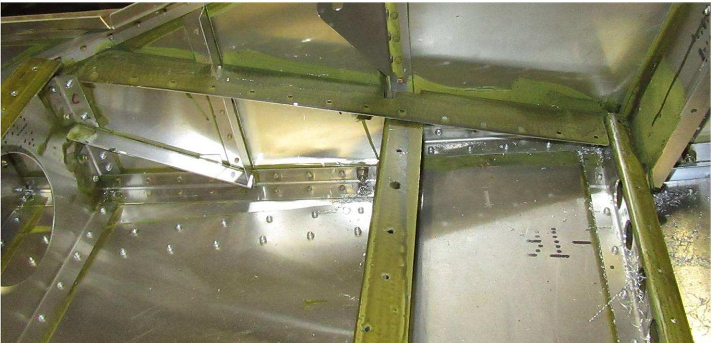
Seat base angle C75F11-7/1 (shown with the channels for the sliding seat option).
