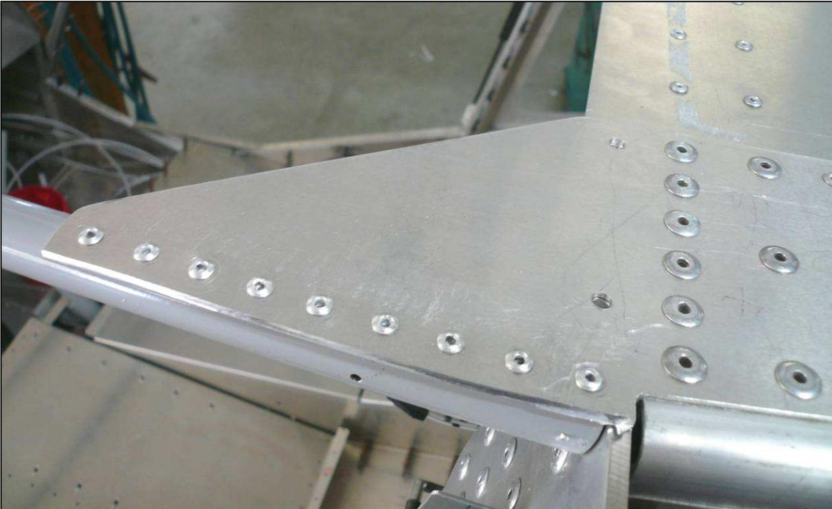
Cleco the aft most hole in the Cabin Frame to the Top Doubler. With a #40 drill bit, back drill through the Top Doubler into the Cabin Frame for the remaining holes and Cleco. Then with a #20 drill bit, expand the holes and Cleco.
