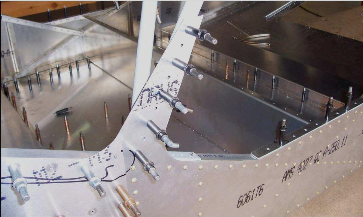
The bottom most hole for the Cabin Side has been predrilled into the Cabin Frame. Cleco the Cabin Side to the Cabin Frame. With a #40 drill bit, back drill through the Cabin Side into the Cabin Frame and Cleco. Then with a #20 drill bit, expand the hole and Cleco.
