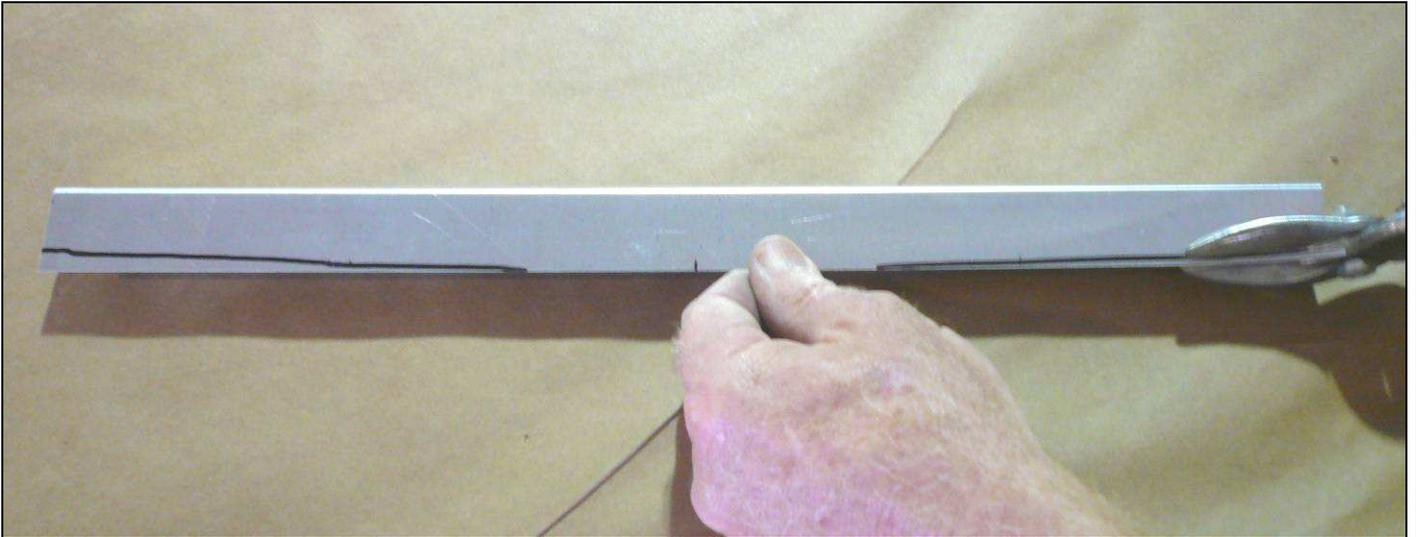
Make a mark at each end of the Angles at the distance measured in the previous step. Make a smooth curve to the center of the Angle from the marks at each end. Trim the Angle along the line to match the curvature of the Side Skin.
