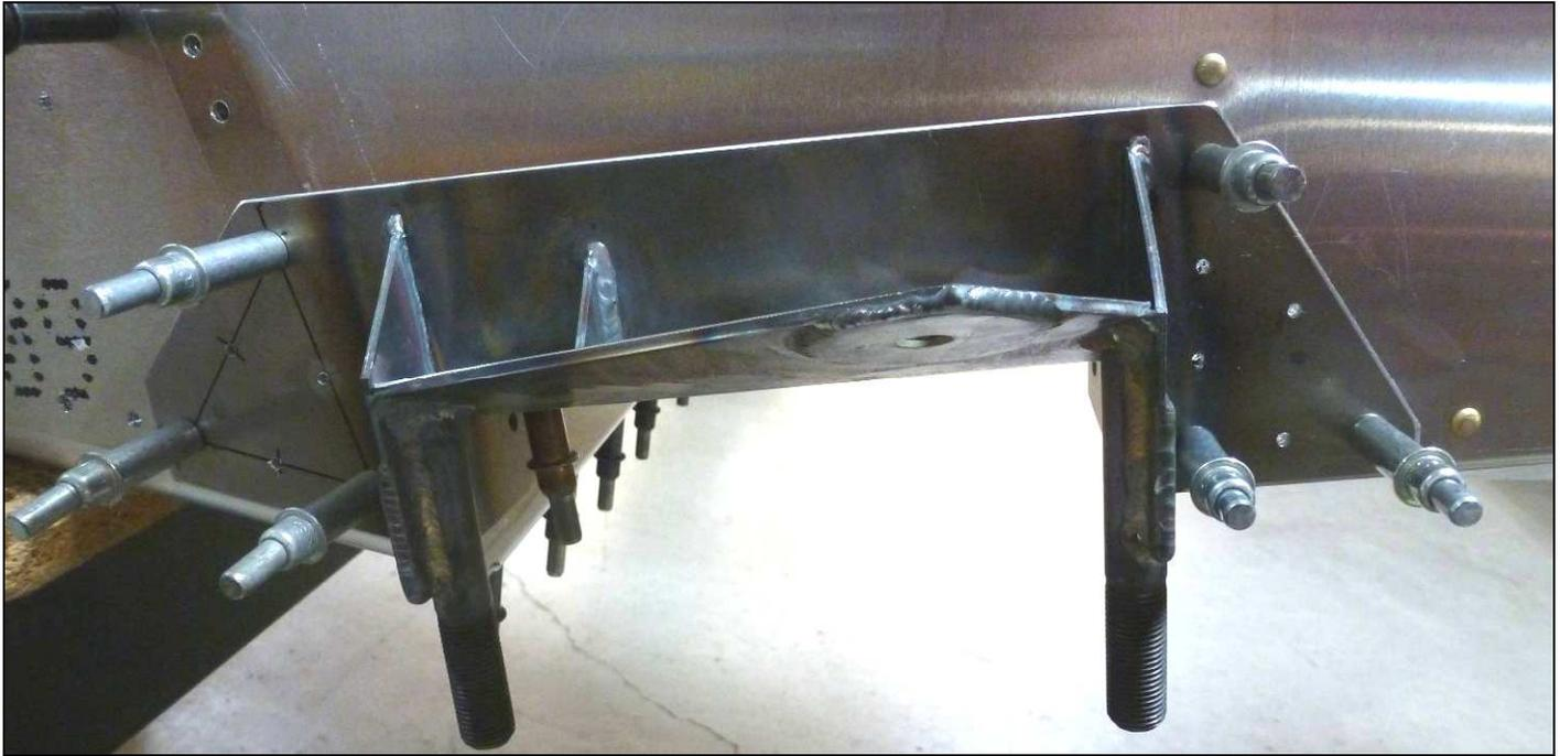
With a #40 drill bit, drill the bolt and rivet locations on the Gear Strut Fitting into the Fuselage and cleco. Expand all the holes with a #20 drill bit and cleco. Expand the 10 holes for the bolts to 3/16", then expand the top hole in the Gear Strut Fitting through the Side Channel to 1/4".
