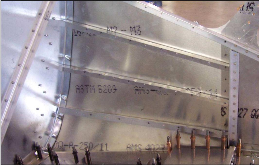
Trim L Angles to fit on the Forward Side Skin. Draw a center line on one flange of L Angles. Position the Angles on the Forward Side Skin so the line is visible through the predrilled holes. Crimp the top flange to match the curvature of the Side Skin. With a #40 drill bit, back drill through the Side Skin into the L Angles and Cleco. With a #30 drill bit, expand the holes and Cleco.
