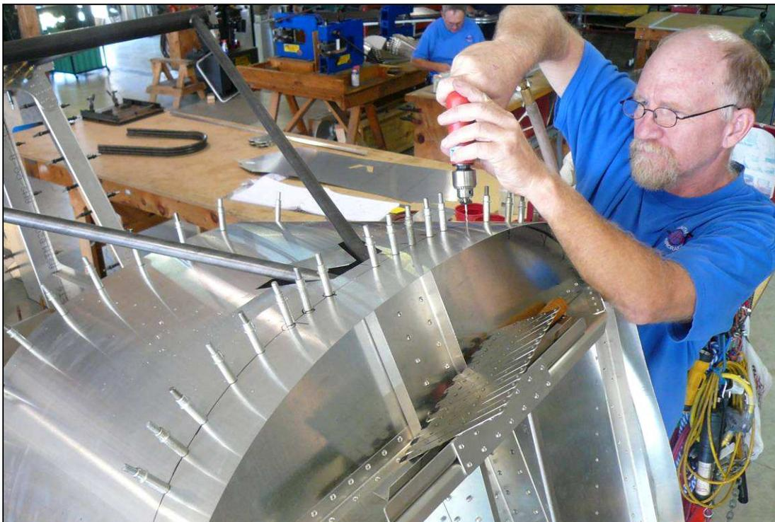
With a #40 drill bit, back drill through the Forward Top Skin into the Firewall. Start in the center and work to each edge. Cleco every hole as they are drilled to pull the Skin tight to the Firewall. Back drill through the Side Skin into the Top Skin and Longerons and Cleco. With a #20 drill bit, expand the holes for the Firewall and Longeron and Cleco. With a #30 drill bit, expand the holes through the Instrument Panel.
