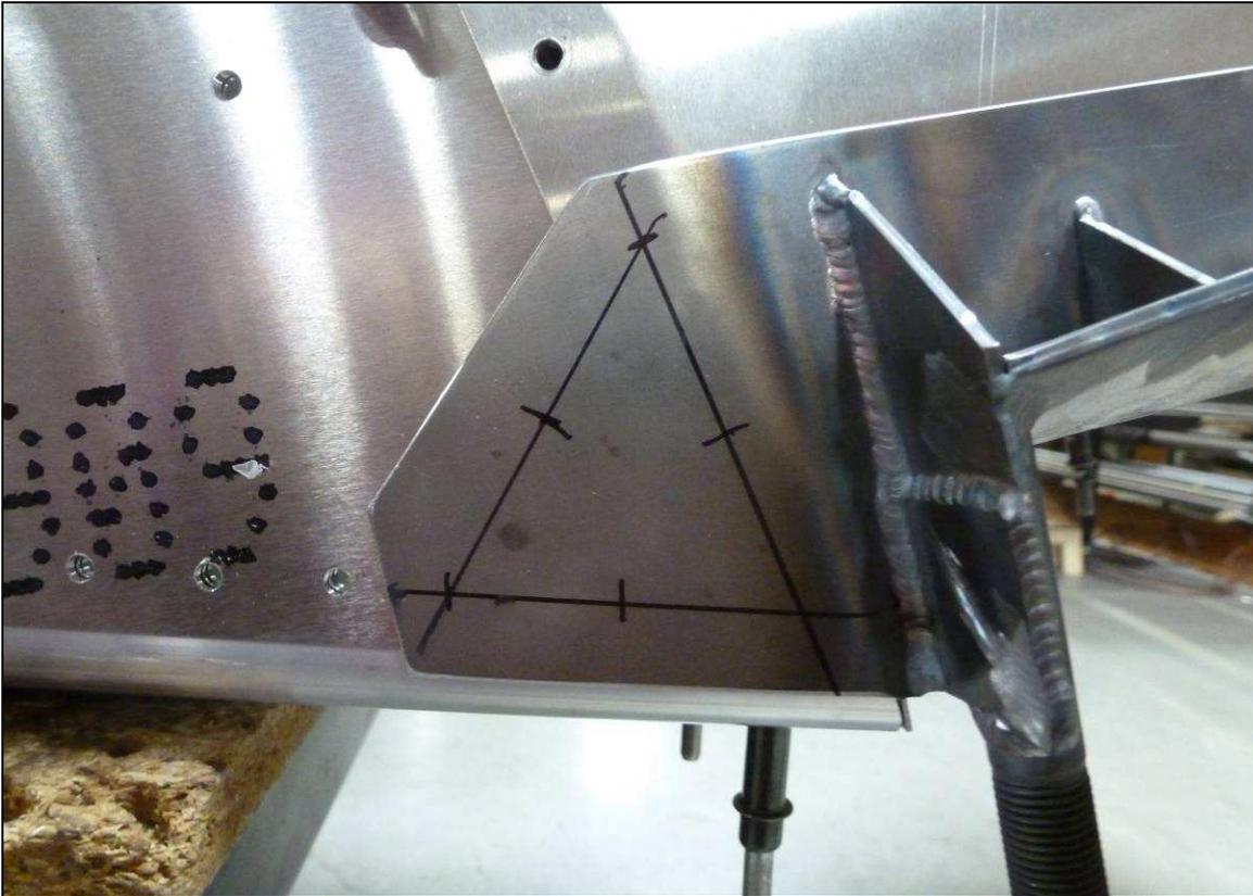
Mark a hole location 10mm from the ends and one half way between. Layout a rivet location 10mm from the edge, half way between the bolt locations.
