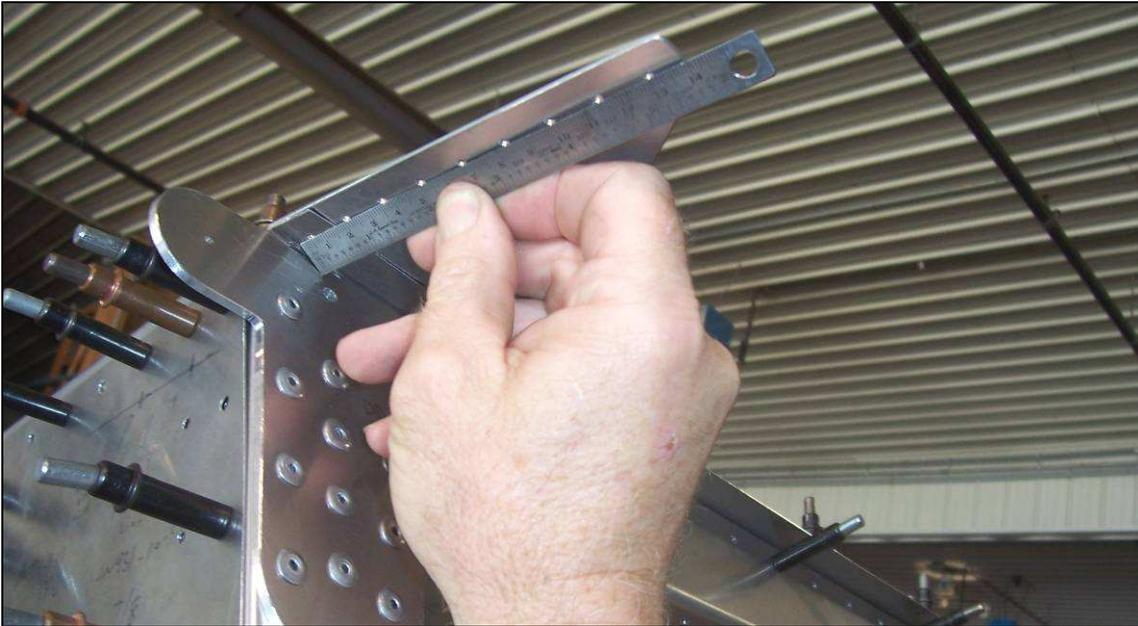
Measure the distance between the Rear Wing Attachment and the first hole in the Top Doubler.
