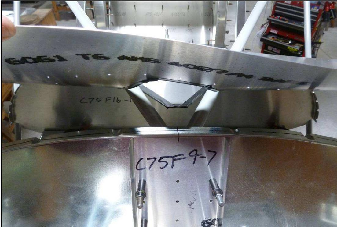
Draw a line centered on the flange of the Firewall. Also make the center of the firewall on the top flange and front of the Firewall.
