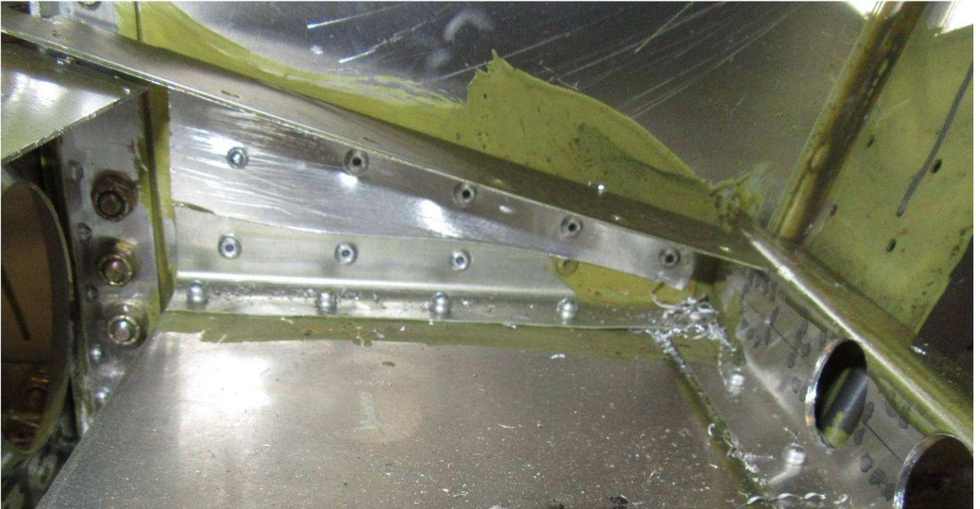
Cut a piece of L angle 150mm long. Mark the center line on one flange. Mark a rivet location 10mm from each end of the L angle, then even space 3 more rivet locations. With a #40 drill bit, predrill the holes in the L angle. Position the L angle on the Gear Channel against the Cabin Side. Back drill through the L angle into the Cabin Side and cleco. Back drill through the Gear Channel into the L angle and cleco. With a #30 drill bit, expand the holes and cleco.
