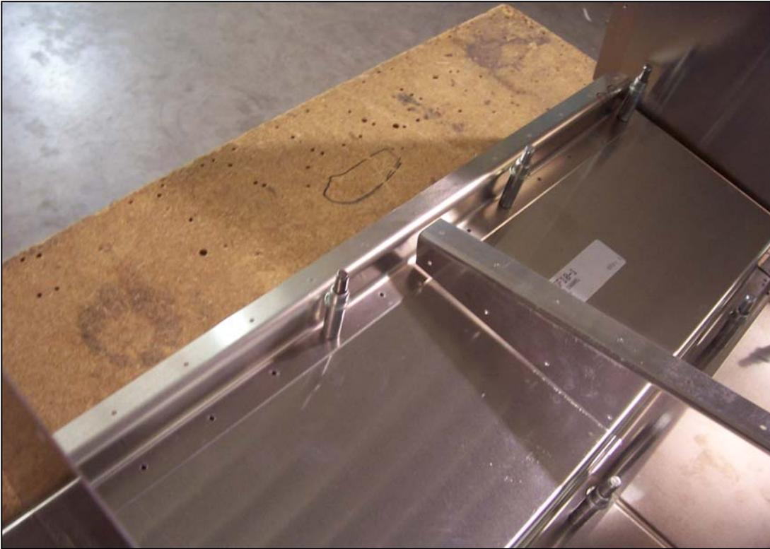
Cleco the Rear Seat Channel to the Gear Channel.
