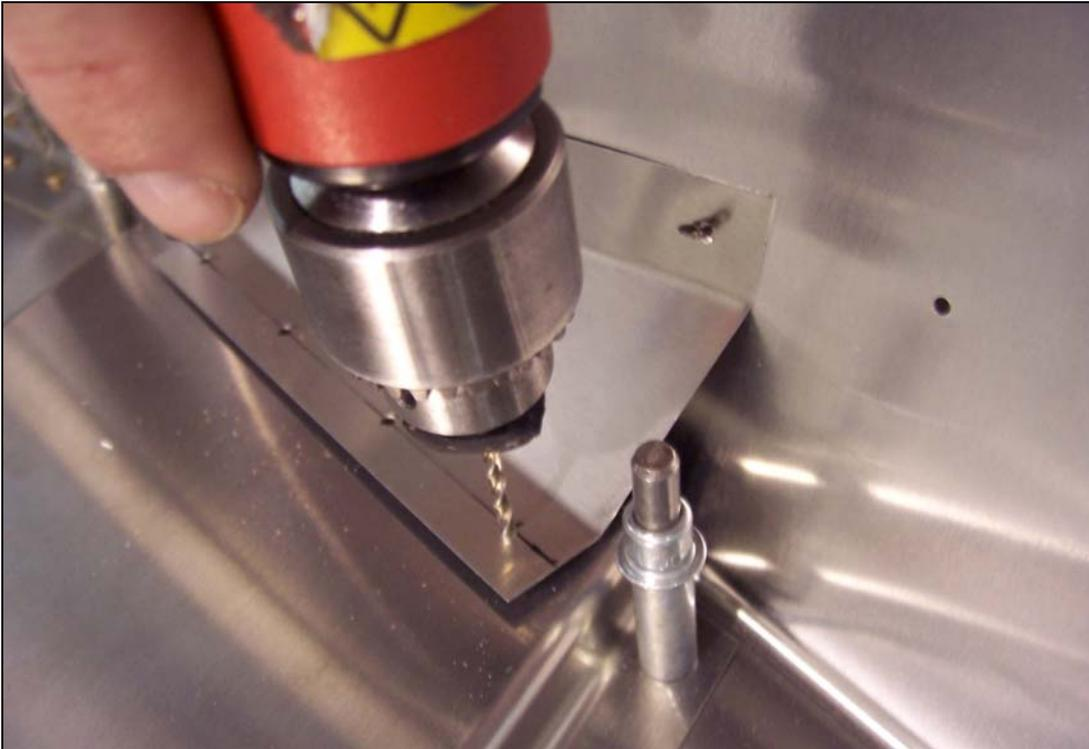
Position the Gusset on the Heal Support against the Forward Side Skin. When the top flange center line is visible through the predrilled holes in the Forward Side Skin back drill through the Forward Side Skins into the Gusset with a #40 drill bit and Cleco. Then back drill through the Gusset into the Heal Support and Cleco. With a #30 drill bit expand the hole in the **BOTTOM** flange only and Cleco.
