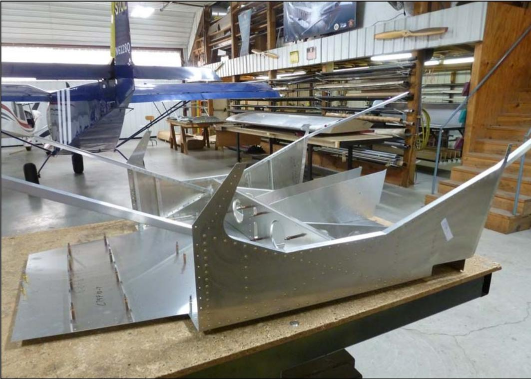
Remove the Cabin Sides from the Rear Fuselage. Cleco the Cabin Sides to the Floor Skin.
