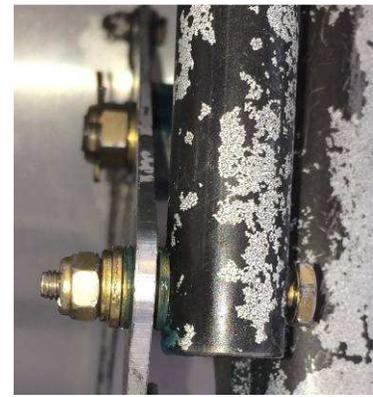
Insert the AN3 bolt through the Elevator control tube , add a ¼" washer, the bellcrank, another ¼" washer, then a 3/16" washer and the castle nut + cotter pin.
