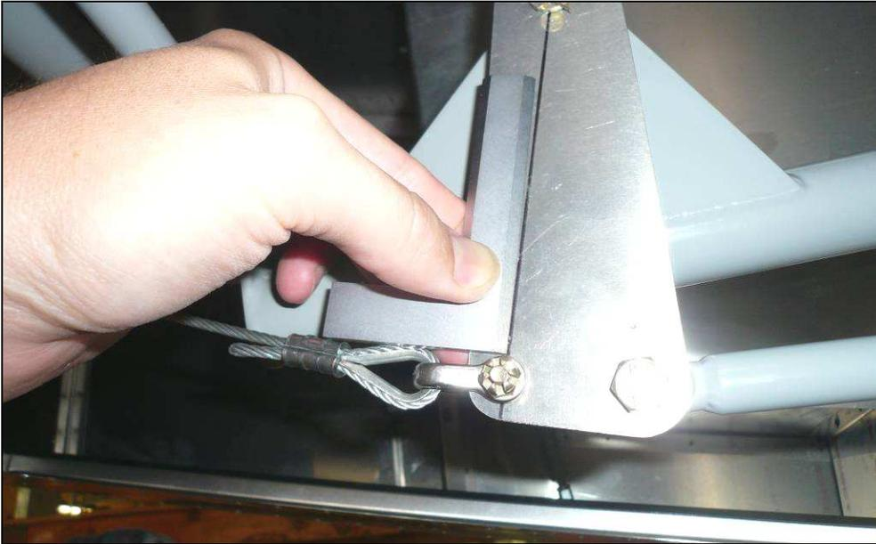
Attach the control cables to the Control Horns on the Elevator. Set the Elevator in the **Neutral** position (the top of the Elevator should be parallel to the top of the Horizontal Stabilizer). When the Bellcrank is in the Neutral position, the cable will be 90 degrees to the line on the Bellcrank. Adjust the cable length and set the Bellcrank in the neutral position.
