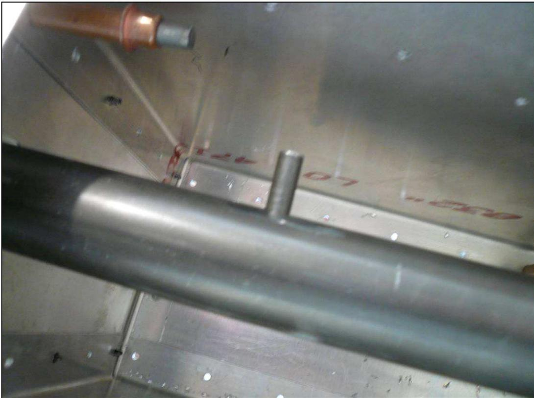
Slide the end of the Bushing into the Torque Tube. The Bushing's outer surface will turn in the bushing welded inside the Torque Tube. Put grease on the outside of the Bushing before final installation.
