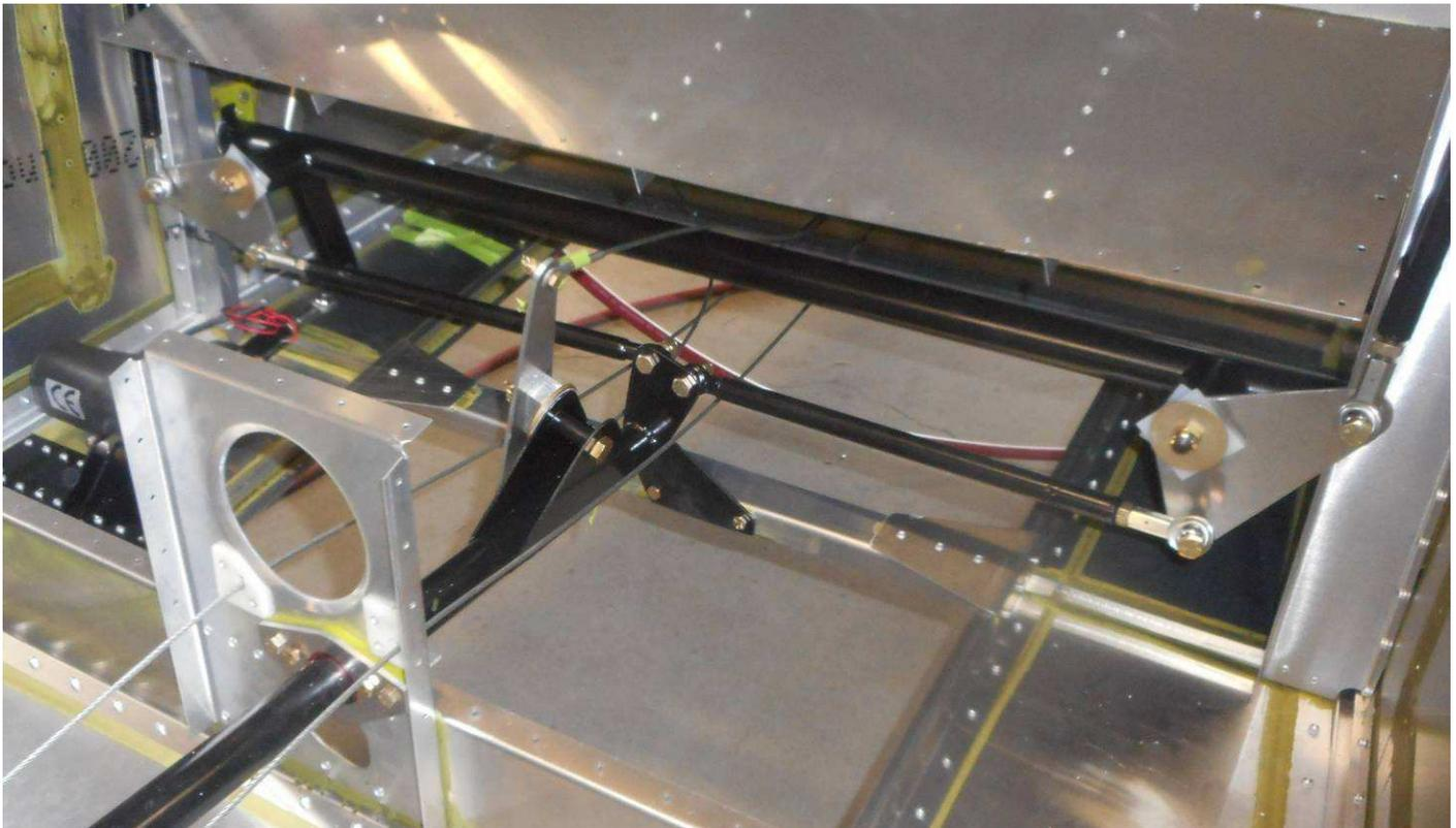
Slide one Bushing on the Bolt, followed by the Rod End on the Control Rod with a second Bushing after it. Install the assembly on the Bellcrank on the Mixer. Don't torque the nut until after the Wings are installed to make adjustments for the Neutral Position of the Flaperons.
