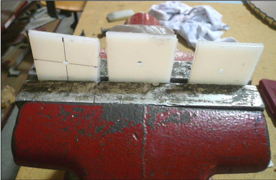
Mark the center of the Flaperon Bellcrank Bearings. With a #40 drill bit, drill a hole in the center of the Bearing. Expand the hole up to 1/2" in steps. It is helpful to clamp the Bearing in a vise to prevent it from spinning while drilling the holes.
