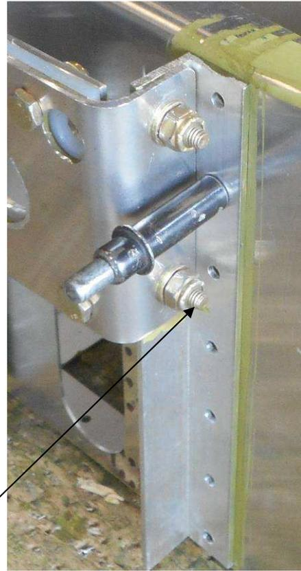
Check that the bolts will not interfere with the rivets
