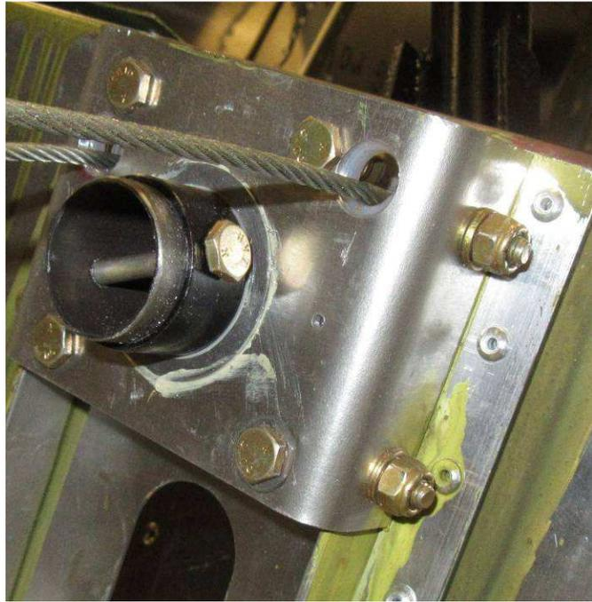
The welded tab on the torque tube make contact with the Bearing support C75F5-1.
