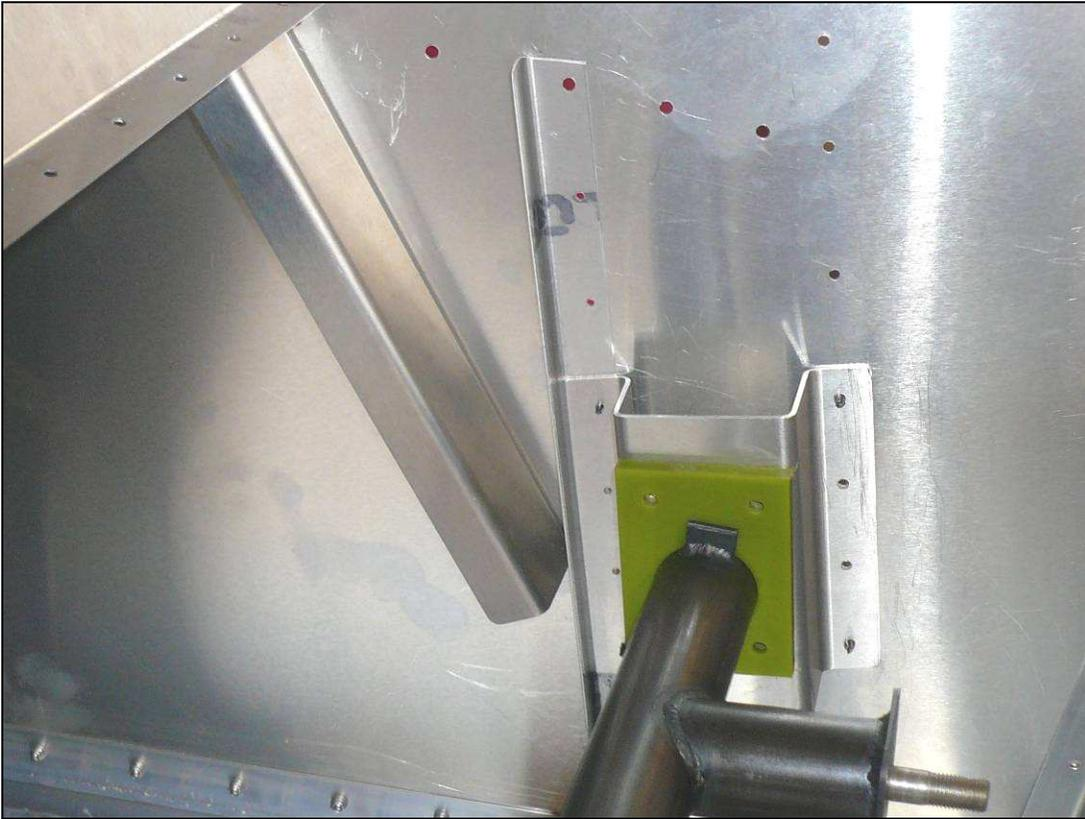
Cut an L angle 303mm long. Position the L Angle against the tab on the Longeron and against the inside of the Bearing Support. Clamp the L Angle to the Bearing Support. With a #40 drill bit, back drill through the Skin into the L Angle and Cleco. Expand the holes with a #20 drill bit and Cleco.
