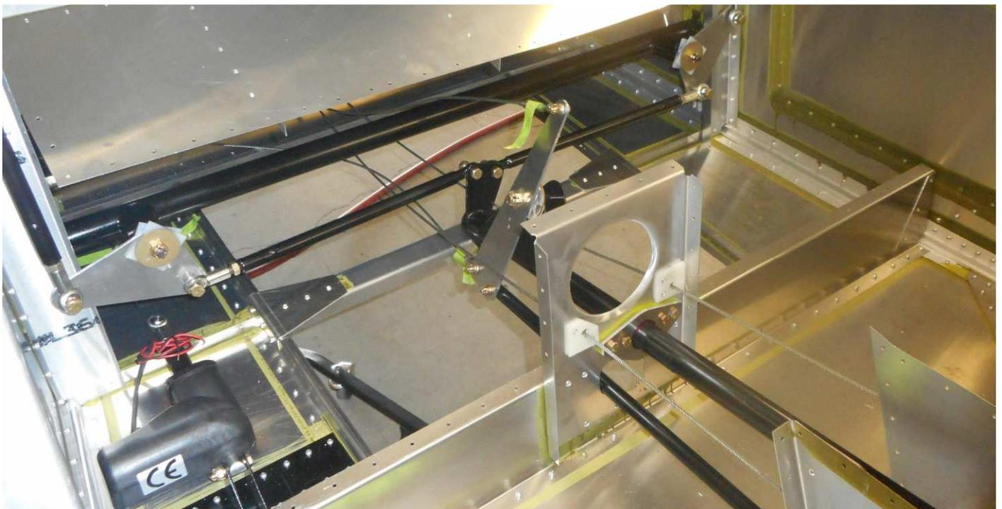
The 15mm x 20mm plate welded on the Torque Tube Bearing is against the Bearing Support (back side)
