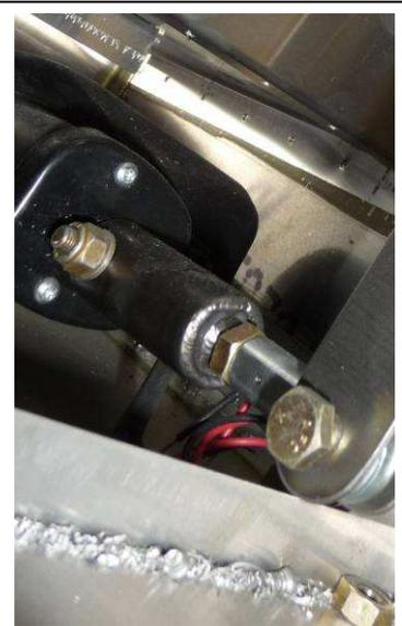
Screw the rod end in all the way as shown in the above photo
