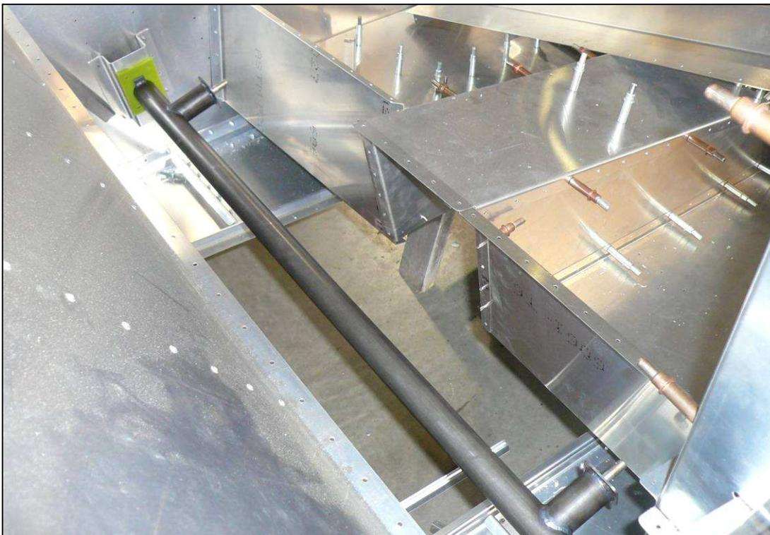
Remove the Baggage Floor from the Rear Fuselage. Slide the Mixer assembly into position in the Rear Fuselage. Cleco the Mixer Bearing Supports to the Side Skins. Wait to expand the holes until the vertical L Angle is installed on the aft rivet line of the Mixer Bearing Supports.
