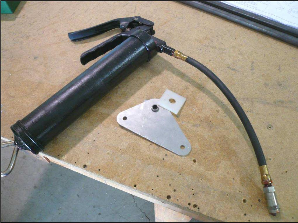
The Flaperon Bushing should turn freely in the Bellcrank, make sure the hole is large enough for it to turn but not be too loose. Grease the outside of the Bushing and the faces of the Bearings that contact the Bellcrank.
