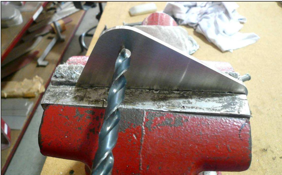
Use a 1/2" drill bit to expand the mounting hole in the Flaperon Bellcrank. See drawing C75-C-1 or 75-CA-1 for the specific hole if in question.
