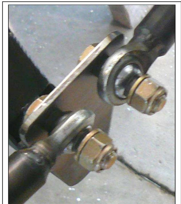
Install the Bolt on the Torque Tube. Slide the first Rod Bushing on the bolt, followed by the Control Rod and a second Bushing. Tighten the nut and properly torque the nut on the bolt.
