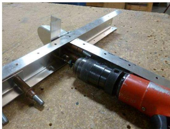
Back drill through the rib and the spar.
