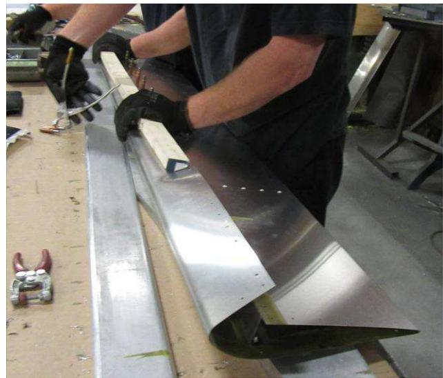
Use a furring strip to bring the Skin around the Nose Ribs and Cleco the Skin to the Spar. This is best done with one person pushing on the furring strip and one person Clecoing the holes. Alternatively, ratchet straps can be used.
