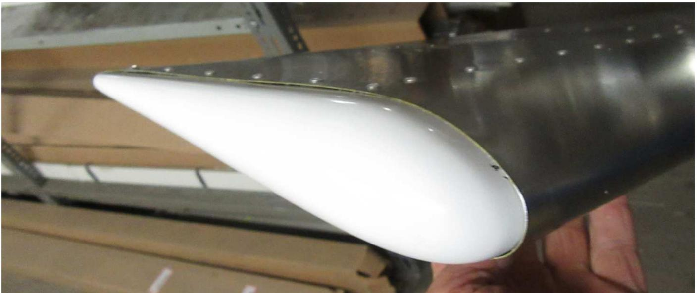
Position for the best fit by closing the gap at the front.
