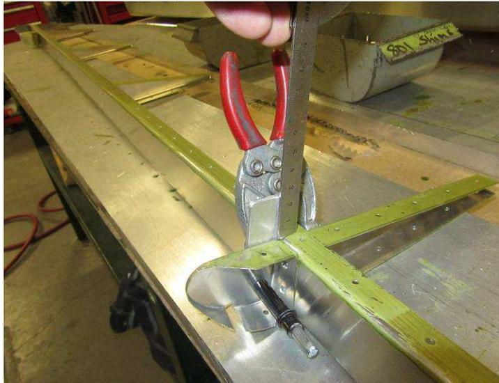
Mark a line at 26mm. Clamp the braret to the spar with the line even with the spar flange.
