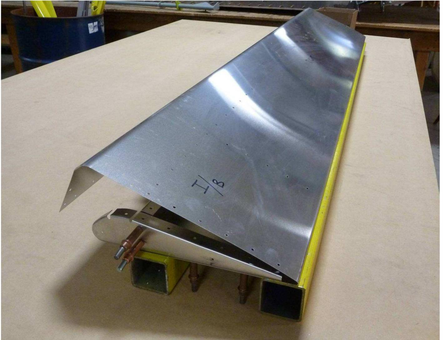
Position the assembly on beams (with clecoes in the bottom side) or on a flat workbench (without any clecoes in the bottom side as shown in the next photo)
