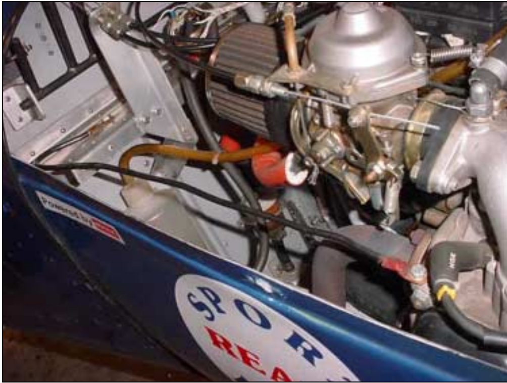
Grounding of engine to airframe (right side of engine)
