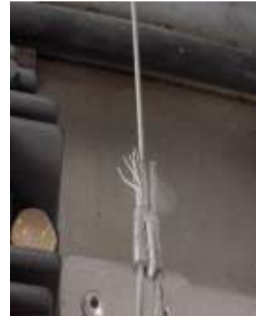
Detail of nico press sleeve used to join left and right throttle cables to the push pull cable.
