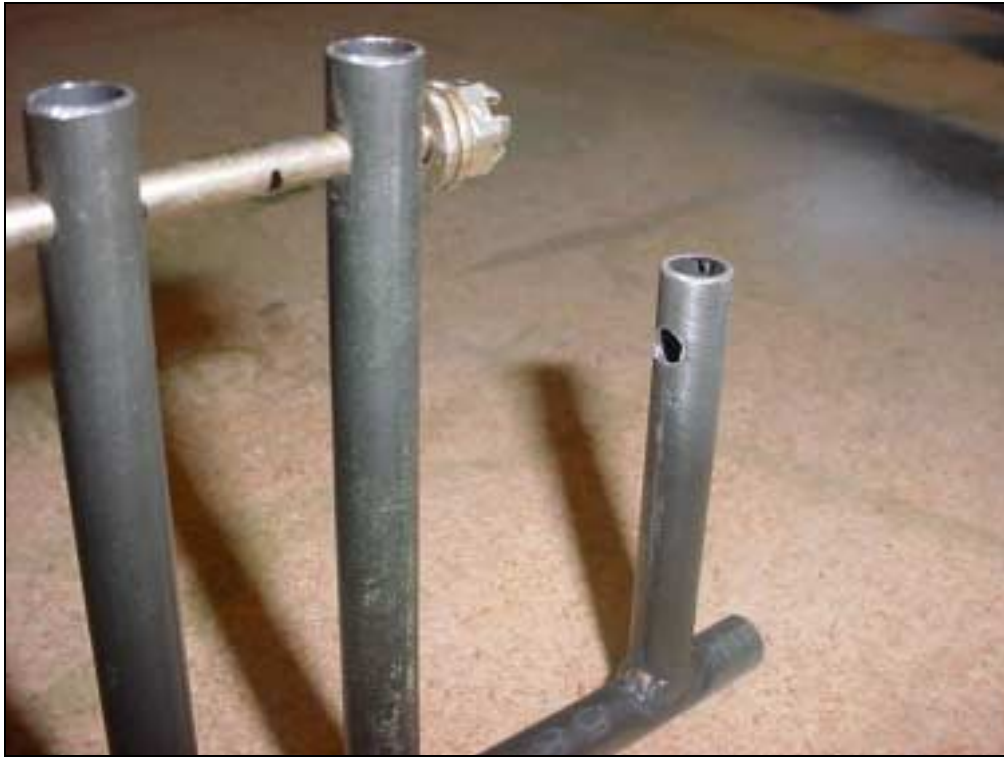
3/16" hole for the throttle rods 7E5-4 in the left and right vertical tube on the bellcrank 7E5-1
