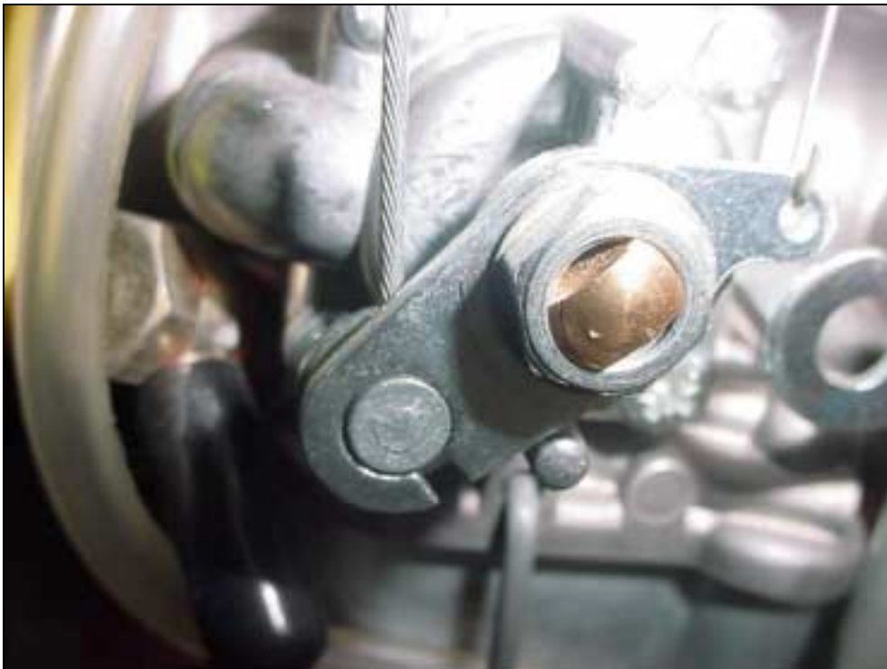
Left Carb: the mark on the choke shaft points towards the cable engagement.
