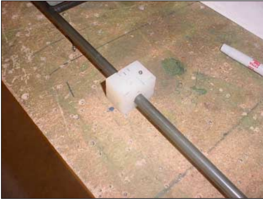
Location of the 3/16" hole Edge distance = 8mm
