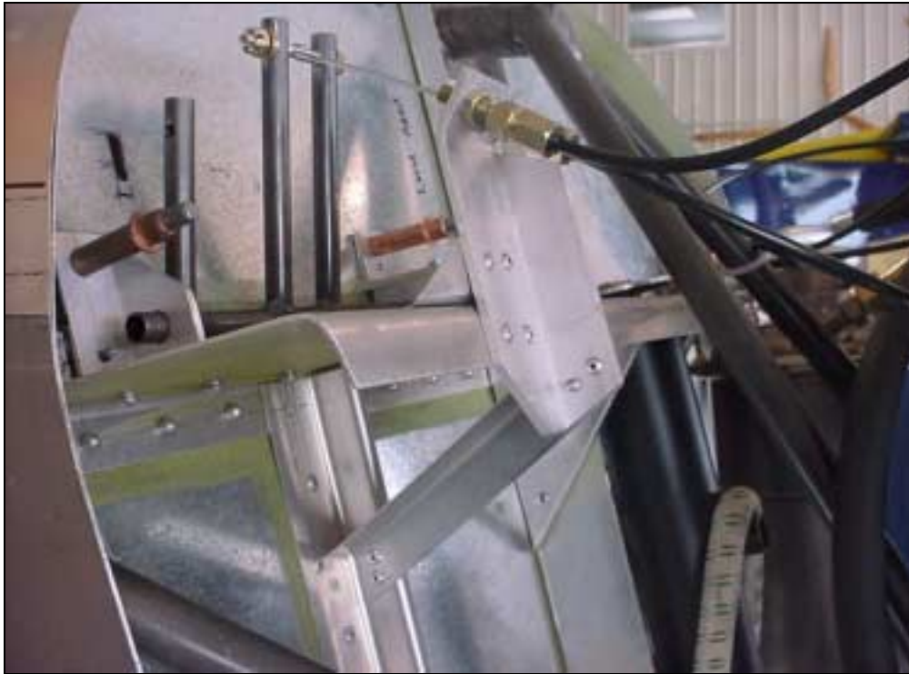
2 RIVETS A4 L angle into 7F7-5
