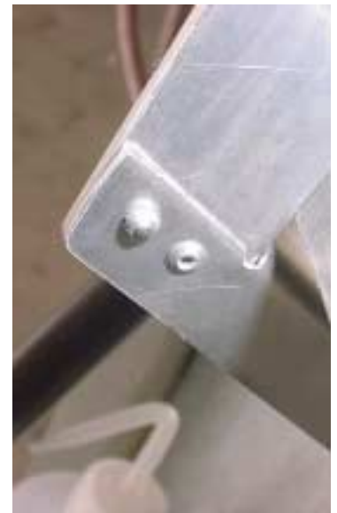
2 RIVETS A4 7E5-3 into L angle
