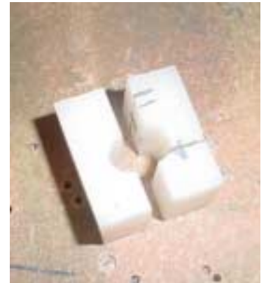
3/8" hole through both blocks
