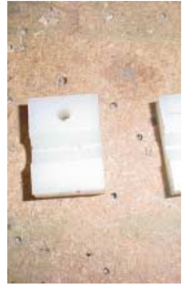
Location of the 3/16" hole Edge distance = 8mm
