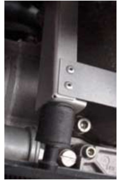
2 RIVETS A5 79-BF into 79-SB
