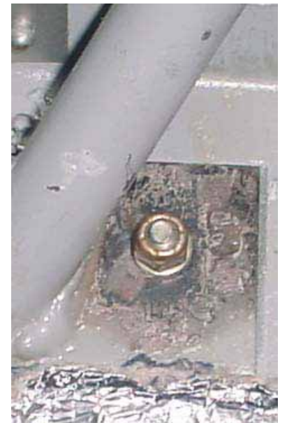
Nylon self locking nut on the cabin side of the firewall.
