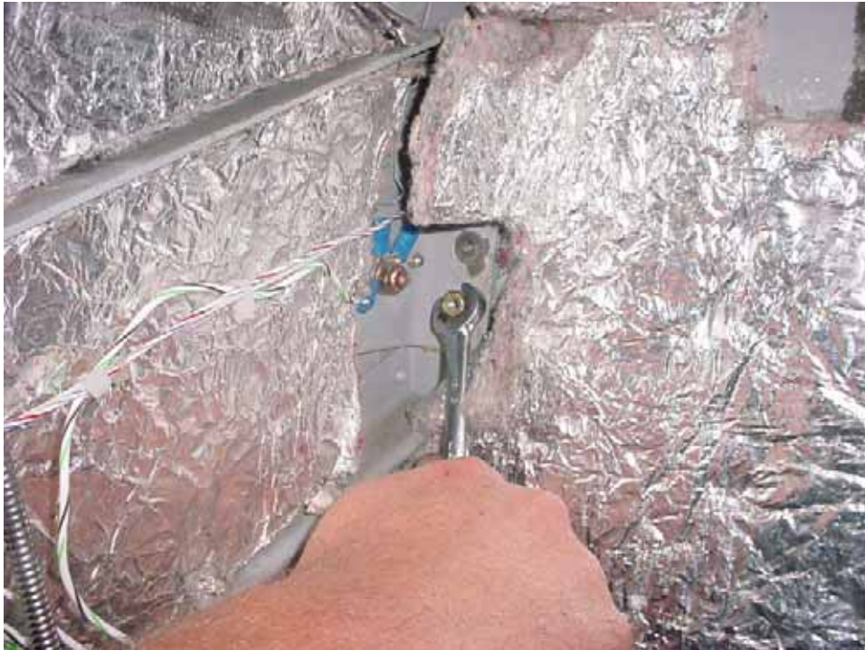
AN3-6A Middle bolt through Steel angle 7F14-5R.
