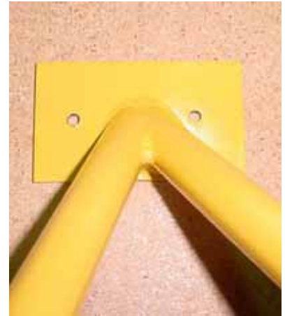
The upper holes are drilled through the firewall and into the cabin frame 7F18-1.
