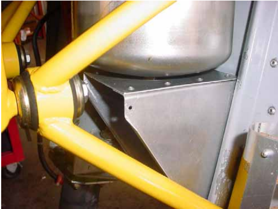
4 rivets 4A top plate to side bracket.
