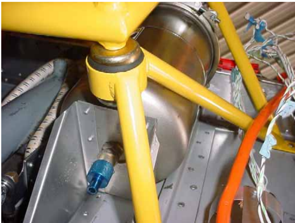
5 rivets A4 through firewall Note: top rivets are pulled from the cabin side.
