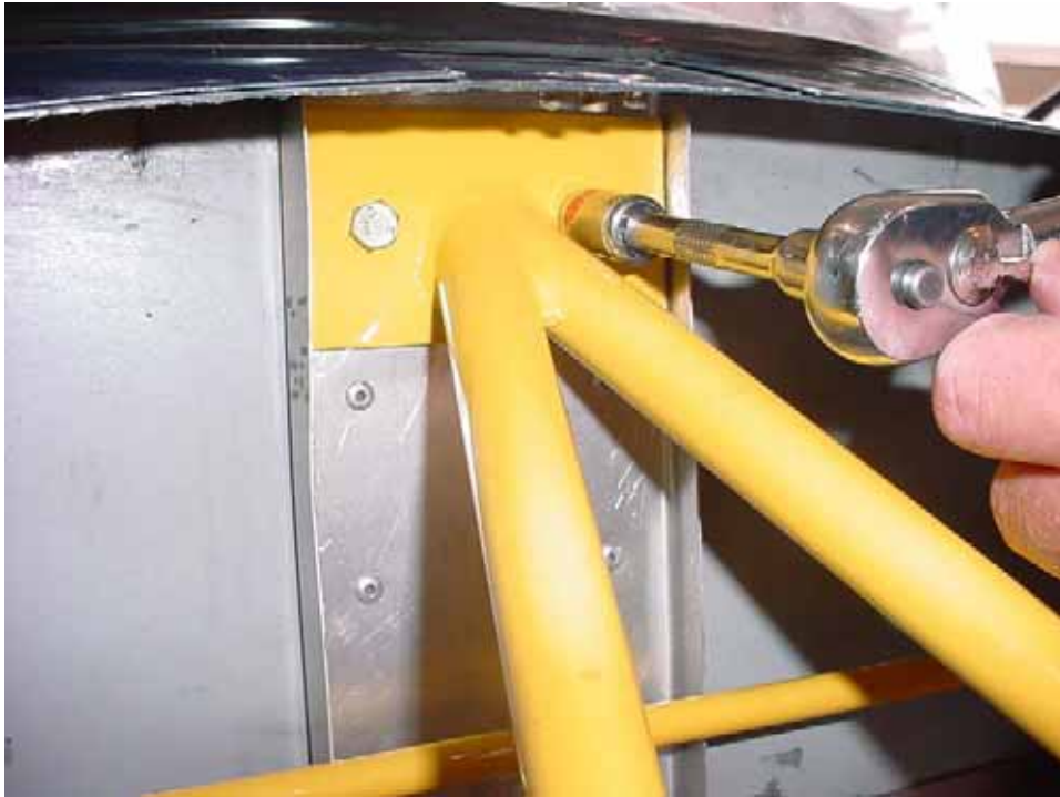
AN3-6A Upper bolts. SUGGESTION: First drill pilot holes and cleco the engine mount to the firewall.
