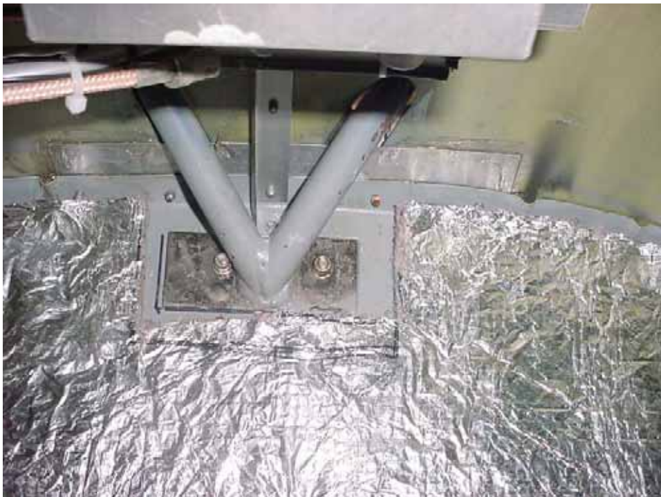
Cabin side view of the firewall and the welded steel plate at the end of the cabin frame 7F18-1.
