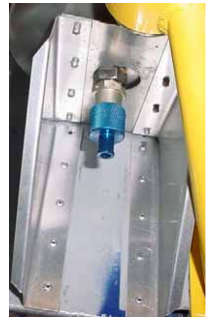
5 rivets A4 through firewall Note: top rivets are pulled from the cabin side.
