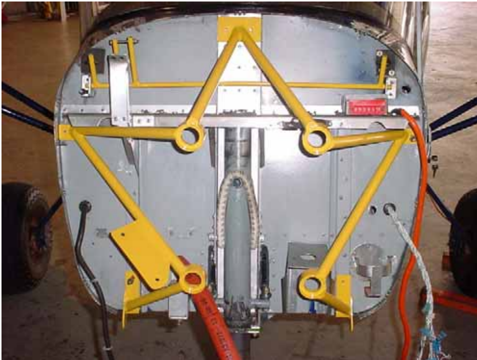
Position the engine mount on the firewall.
