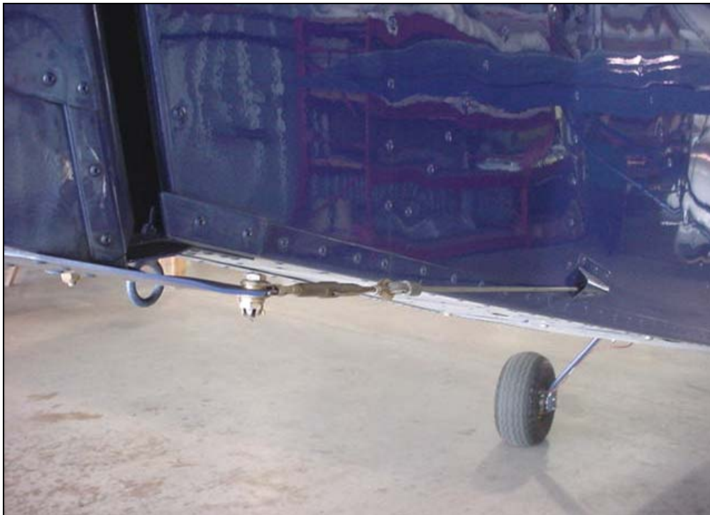
Rudder Horn 7R2-3, the legs are bent down
