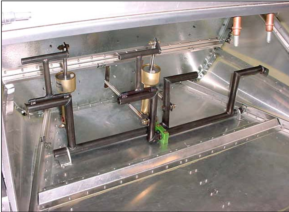
Dual Rudder Pedals with toe brakes on pilot side
