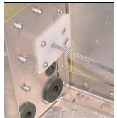
Fairlead 7C5-1A riveted on back side of 7F11-1
